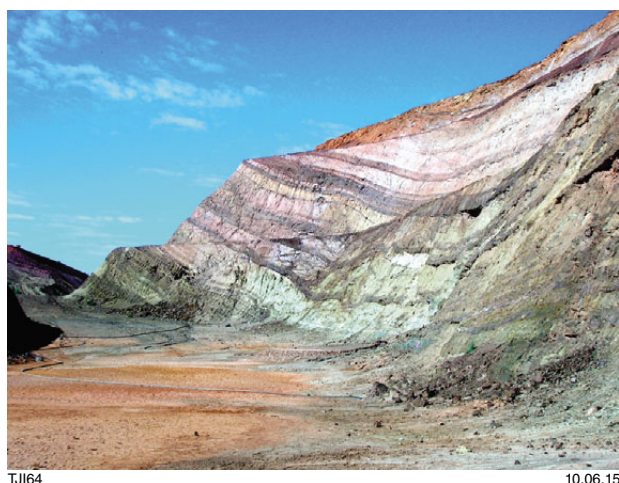
Figure 3. Photograph looking south in the Windimurra vanadium pit showing moderately west-dipping layers of magnetite (dark layers) hosted in magnetite-bearing leucogabbro (pale layers) of the upper zone of the eastern lobe. Pit wall is 30 m high. Note the multiscale cyclicity of mafic and felsic layers creating a heterogeneous rock volume on a centimetre-to-decametre scale.
