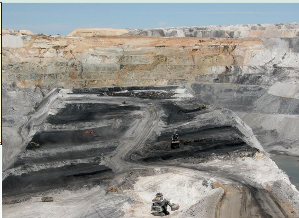
Figure 31. Multiple seam mining of the Muja Coal Measures, Collie Coalfield (from Millar et al., 2011, fig. 6); excavators are 7 m high. The Collie Sub-basin is an outlier of the southern Perth Basin
