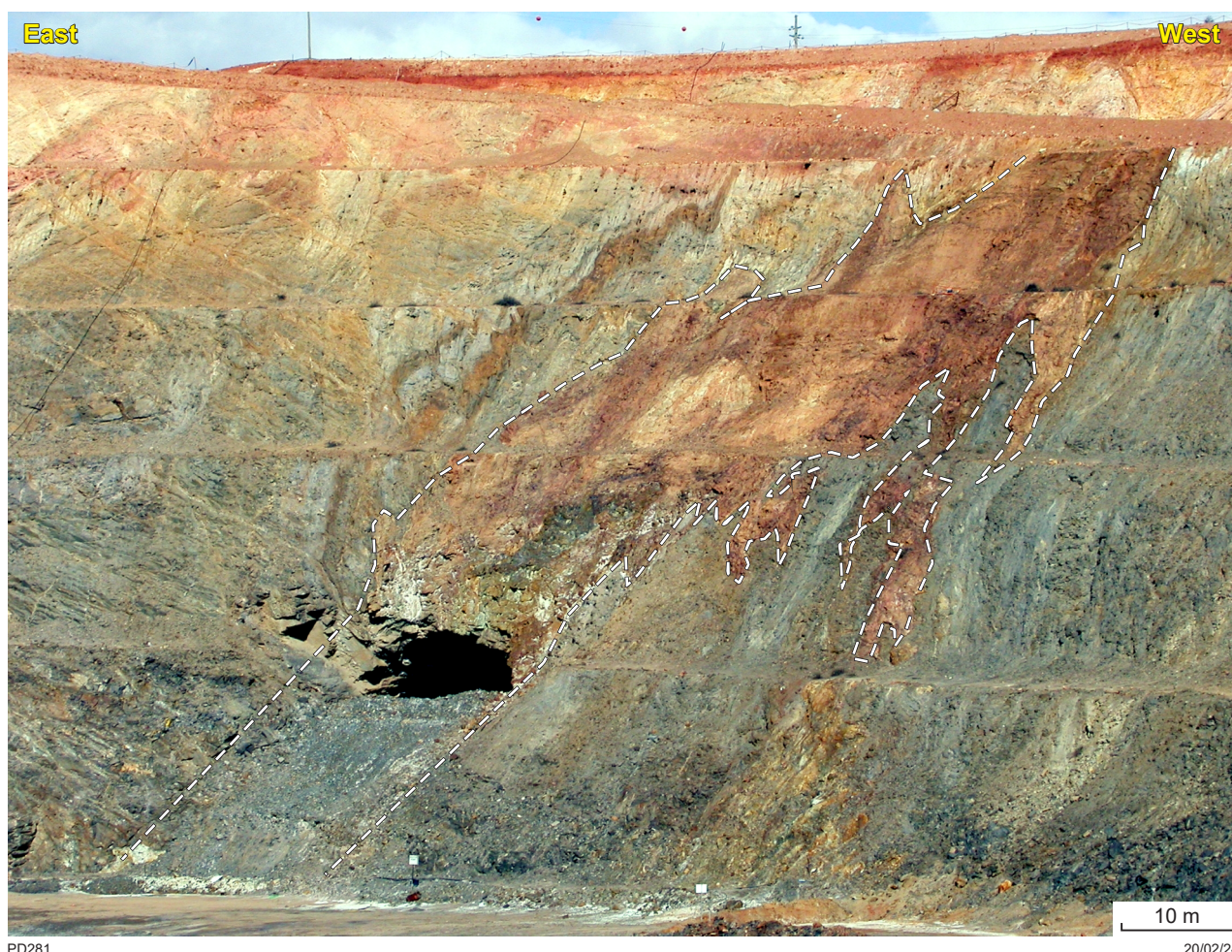
Figure 9. Weathered massive sulfides in folded felsic volcanic country rock, exposed in the southern wall of the Rocky's Reward pit
