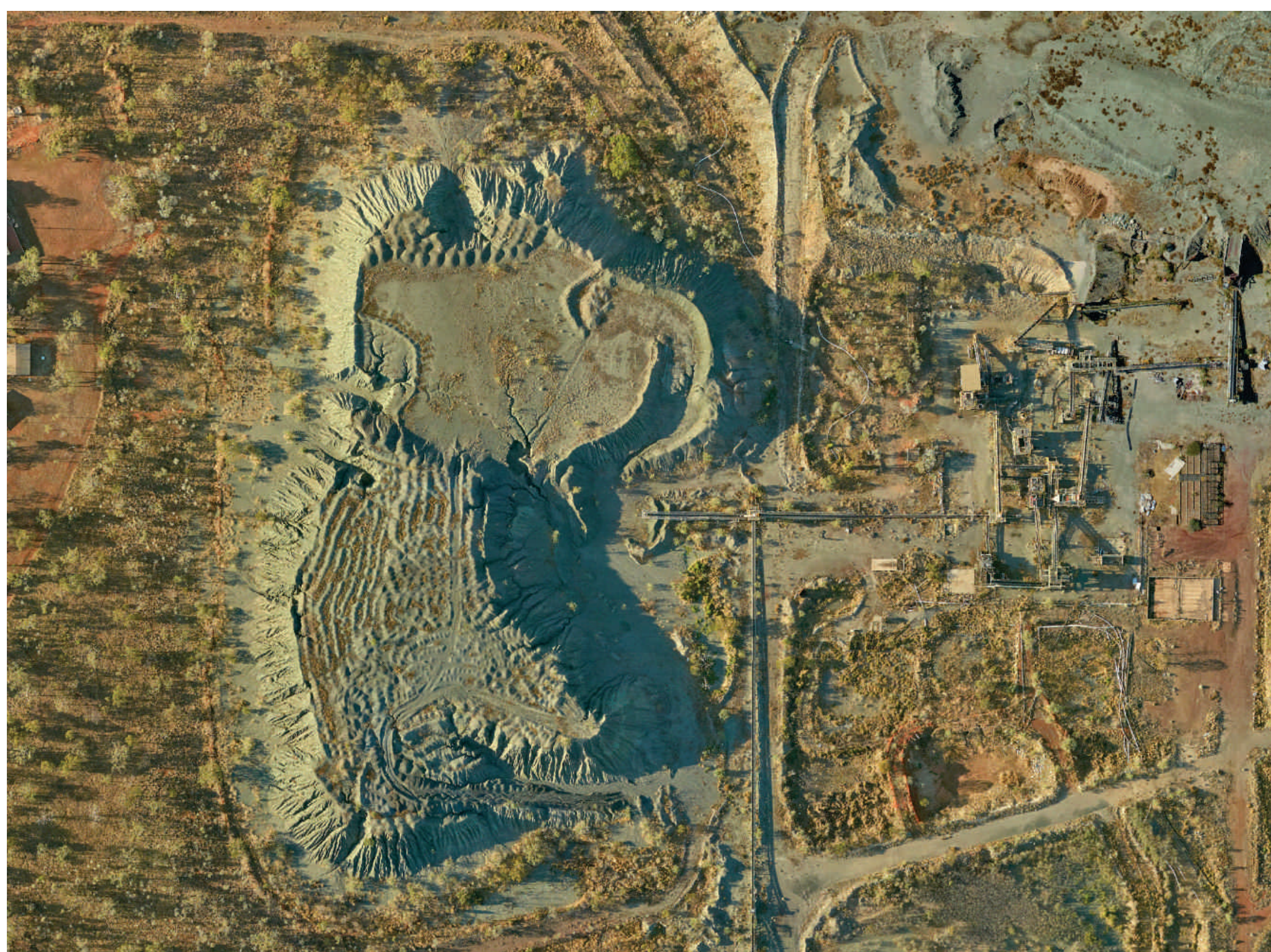
E9 Noise Bund indicating significant landform erosion
