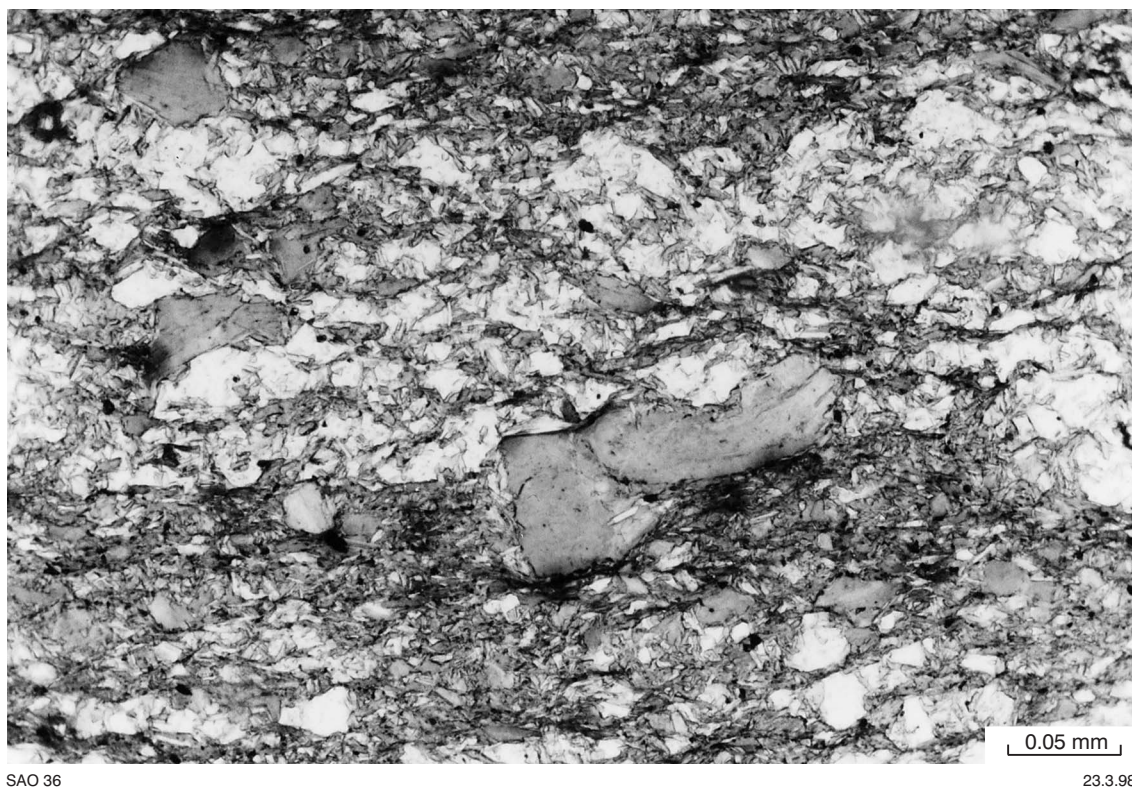
Figure 6. Photomicrograph of chloritic siltstone from the Beatty Park Member comprising quartz, chlorite, and muscovite. Plane-polarized light
