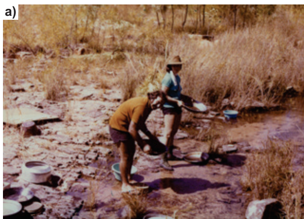
Figure 5. Examples of sampling methodologies used in Western Australian diamond exploration: a) Maureen Muggeridge and Vince Vincello taking alluvial samples at Pteropus Creek, North Kimberley in 1976. The pans and sieves used to screen the samples are evident in the photograph, which also shows the low-energy drainage that often provides challenges to identifying well-sorted trap sites. Photo: DC Lee (digital enhancement: S Dowling); b) tracked drilling vehicle being offloaded in 2013 into the field in the North Gibson Desert west of Lake Mackay (Webb kimberlite project). The vehicle is capable of conducting drilling operations in areas of heavy sand cover and hauling support equipment. Photo: TH Reddicliffe
