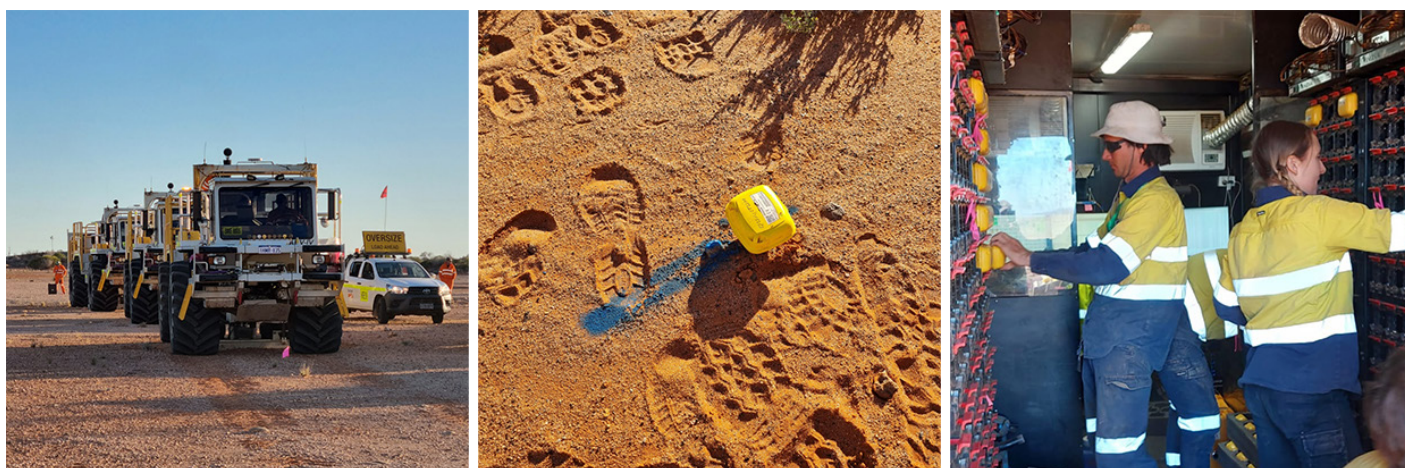
Figure 3. Seismic survey; vibrator trucks (left); geophone in position (centre); downloading and recharging geophones (right). Photos courtesy HiSeis Pty Ltd
