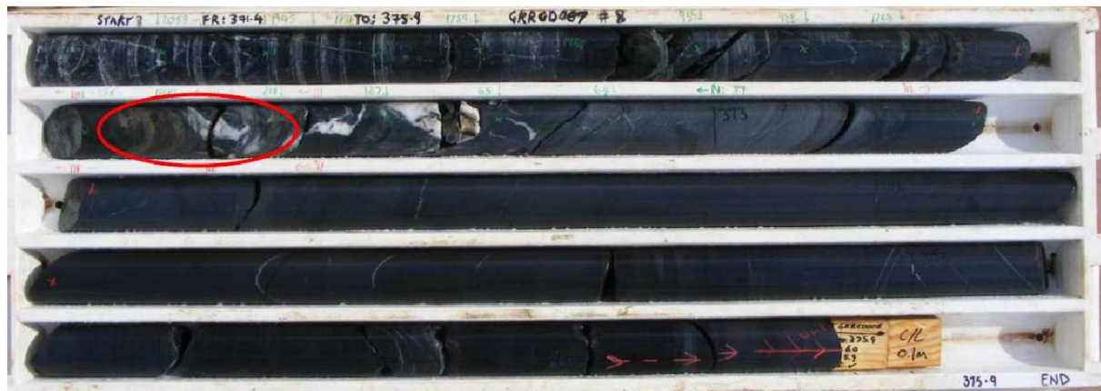
Figure 4. GRR007 core photo: Ni sulphides (red) and basal ultramafic contact with the footwall dacitic unit.
