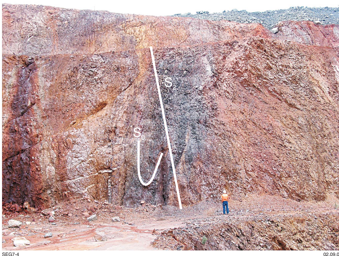
Figure 4. Wall at the southern end of the Super Pit, looking south. Black Flag Group (dark) forms the core of the Lake View Syncline flanked on either side by Golden Mile Dolerite (orangish-brown). The north-northwesterly trend of the regional foliation is highlighted ( S_2 ) and clearly overprints the syncline
