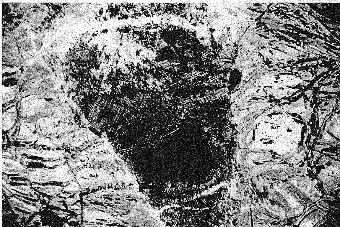
Plate 6B Another view of the sample clearly showing reticulate cleavage textures preserved by Fe - oxide inclusions in the dark brown orthopyroxene - bronzite (bz) phenocryst within the serpentinised (antigorite - ant) adcumulate olivine host. Crossed polars. Field of view - 1.8 mm.
