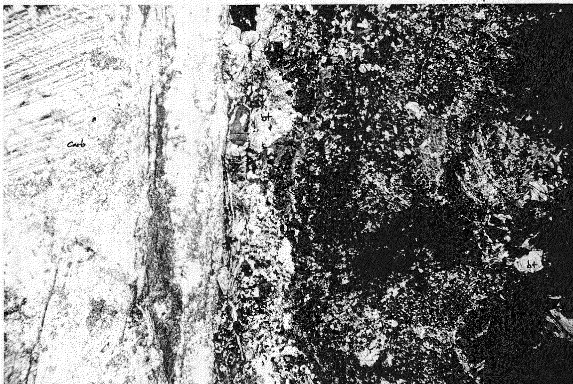
Plate 5A Sample CDD - 01 578.2 m showing the contact between the carbonatite vein and the serpentinised clinopyroxene adcumulate host. Platy biotite has developed along the vein selvage. The ultramafic host contains abundant Fe - oxide inclusions (opaque) and has preserved the closed packed polygonal outlines of original adcumulate clinopyroxene. Crossed polars. Field of view - 3.6 mm.
