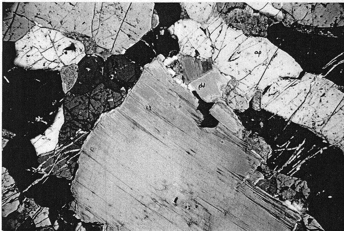
Plate 1B Another view of the sample phlogopite (phl - coloured) enveloping anhedral apatite within the carbonatite vein. Carbonate (carb) occurs interstitially. Crossed polars. Field of view - 3.6 mm.
