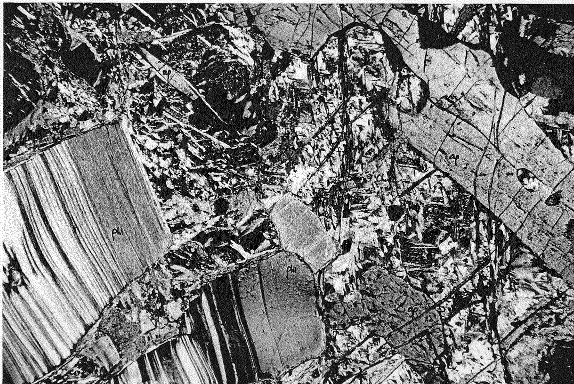
Plate 1A Sample CDD - 01 393.0 m showing platy phlogopite (ph) occurring in a serpentine - minor carbonate (carb) matrix. Biotite is interlayered with chlorite (chl) as a stress - induced retrograde alteration phase. Bladed apatite (ap) occurs within the fibrous chrysotile (chy) matrix. Crossed polars. Field of view - 3.6 mm.
