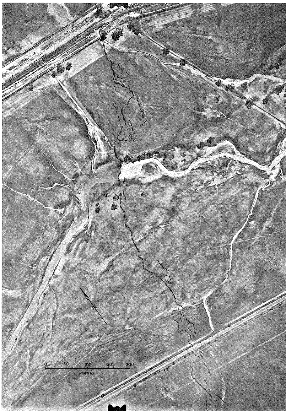
15. A small stream, west of Meckering, dammed by the Meckering Fault. The stream flows east and on the uplifted block the stream bed has dried out (air photo W.A. 1112, 5150).
