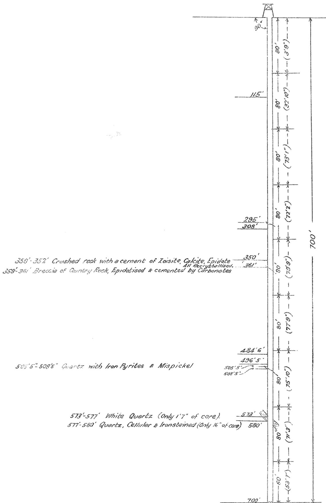
Figures in brackets indicate the length of core recovered from the corresponding section of boring.
