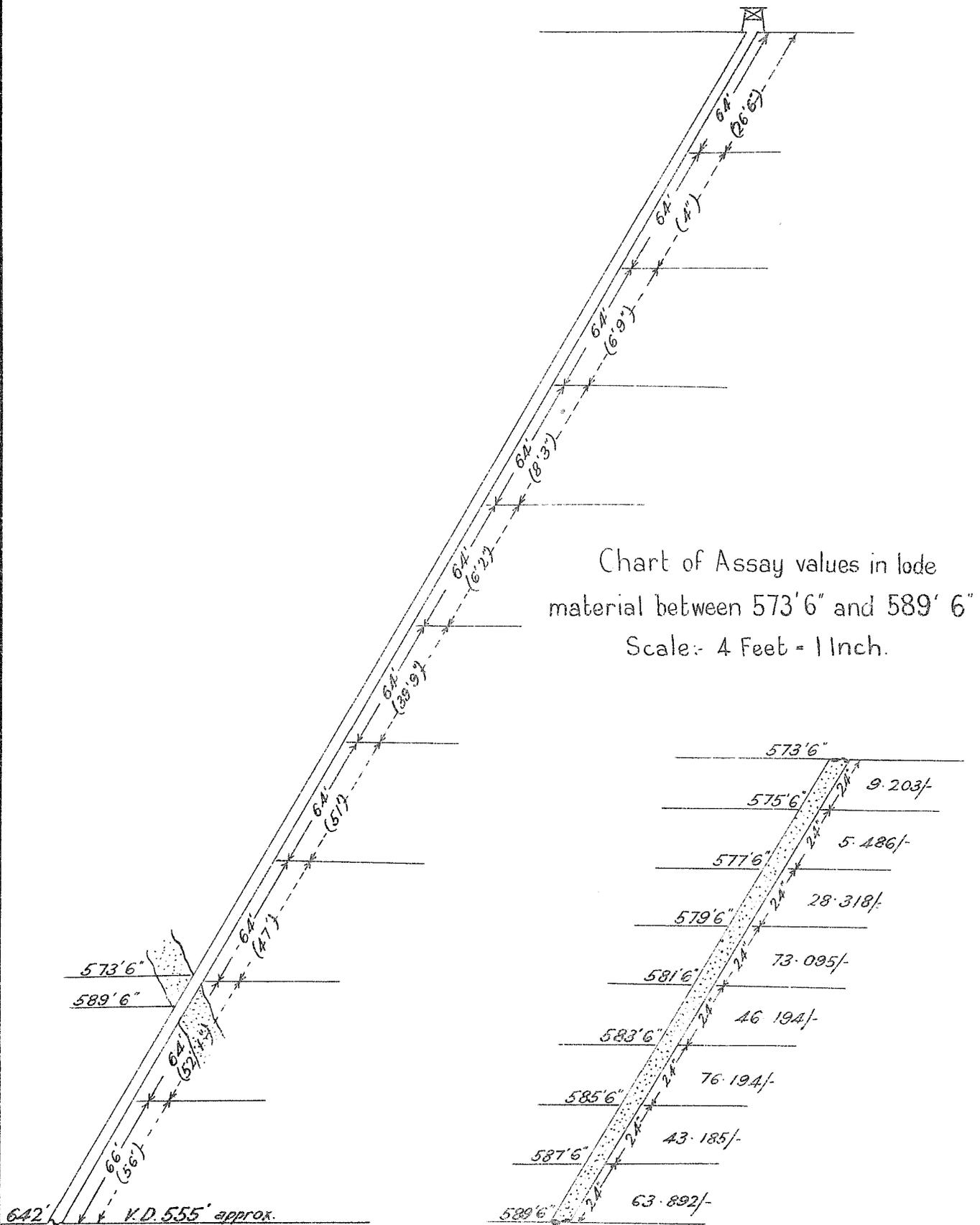
The figures in brackets indicate the length of core recovered from the corresponding section of boring.
