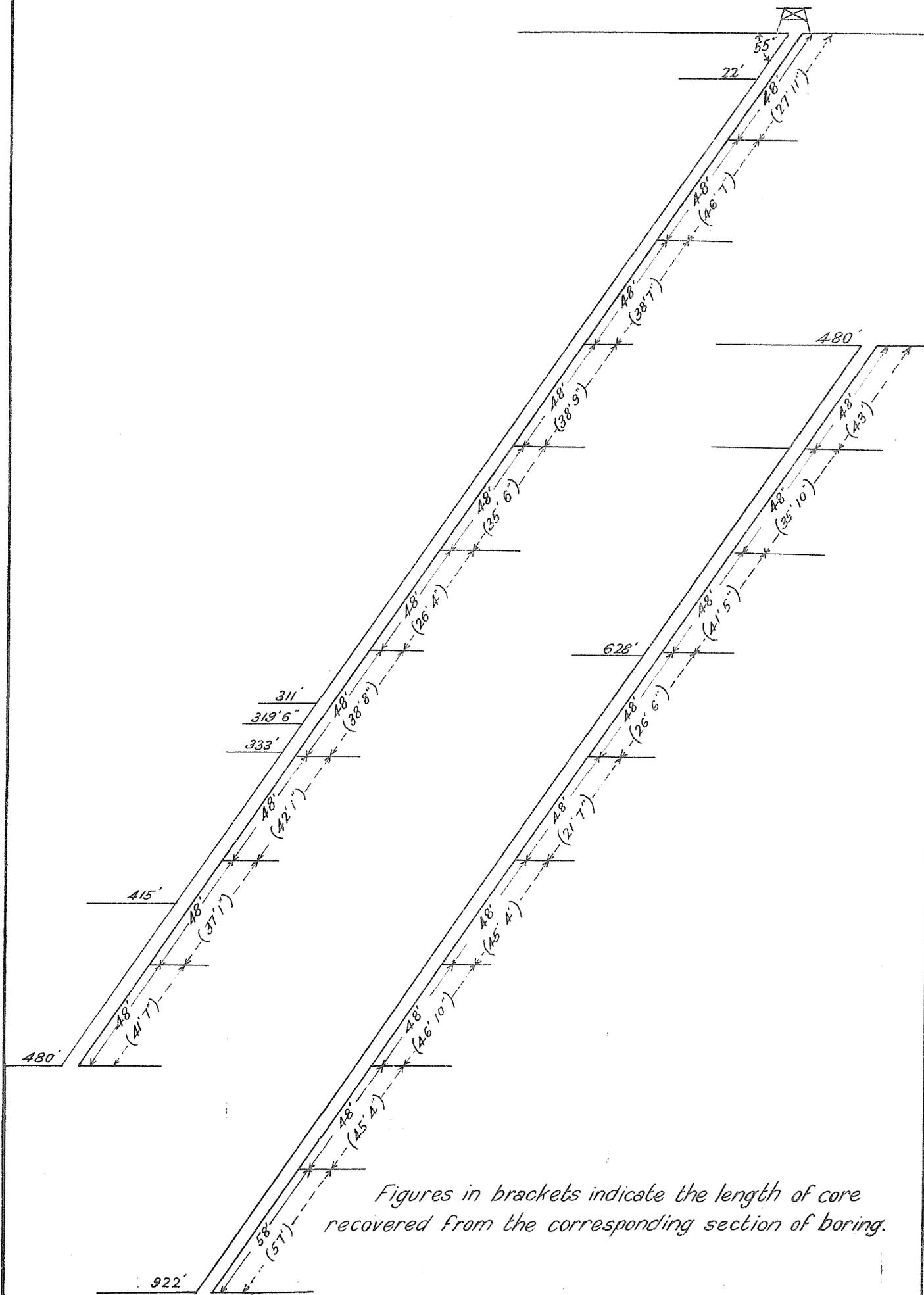
*Figures in brackets indicate the length of core recovered from the corresponding section of boring.*
