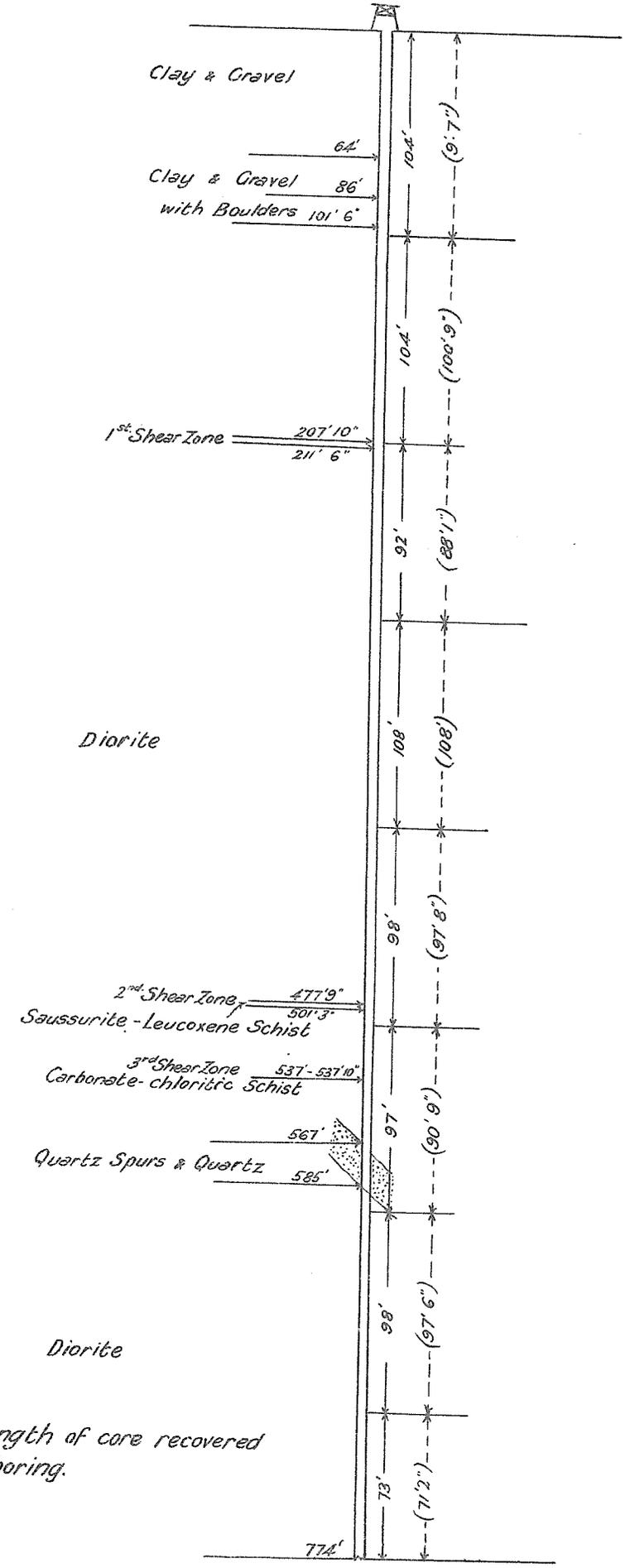
Figures in brackets indicate the length of core recovered from the corresponding section of boring.
