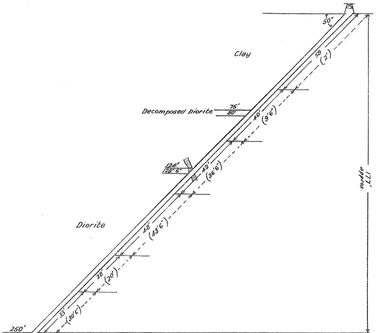
*The Figures in brackets indicate the length of core recovered from the corresponding section of boring.*
