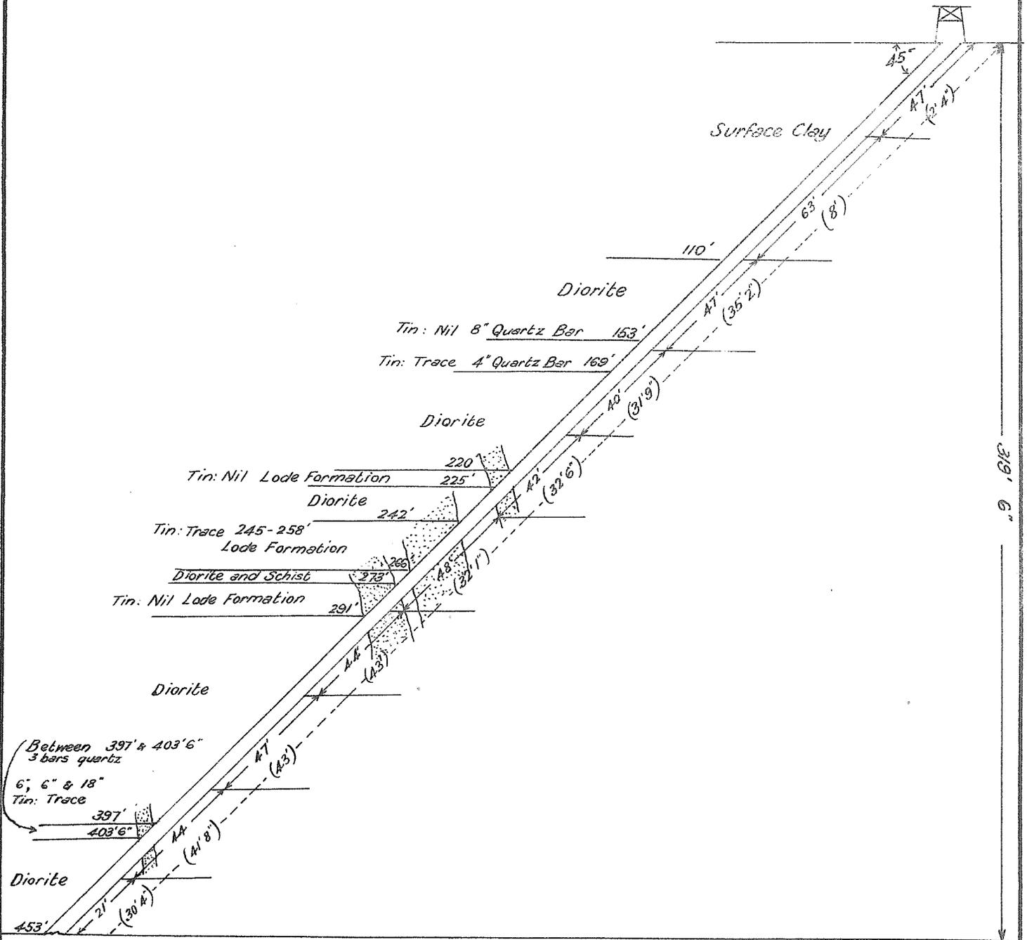
Figures in brackets indicate the length of core recovered from the corresponding section of boring.
