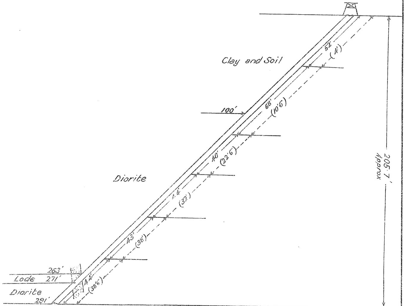
Figures in brackets indicate the length of core recovered from the corresponding section of boring.
