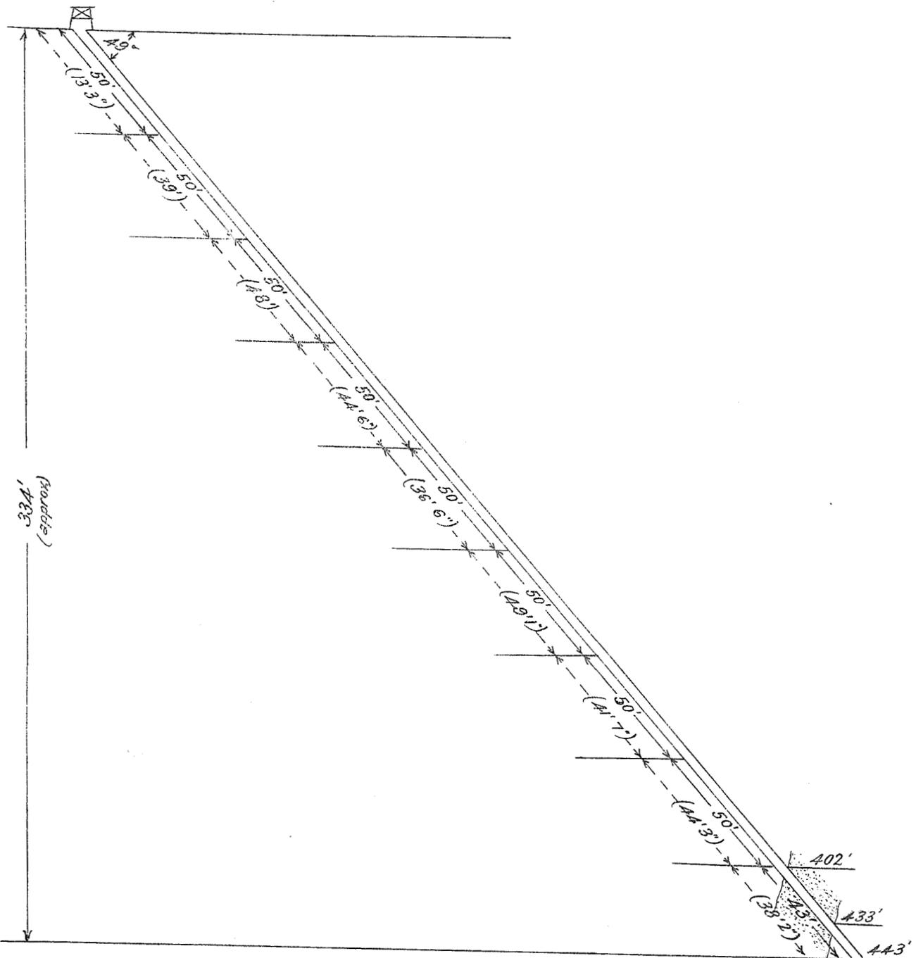
*Figures in brackets indicate the length of core recovered from the corresponding section of boring.*
