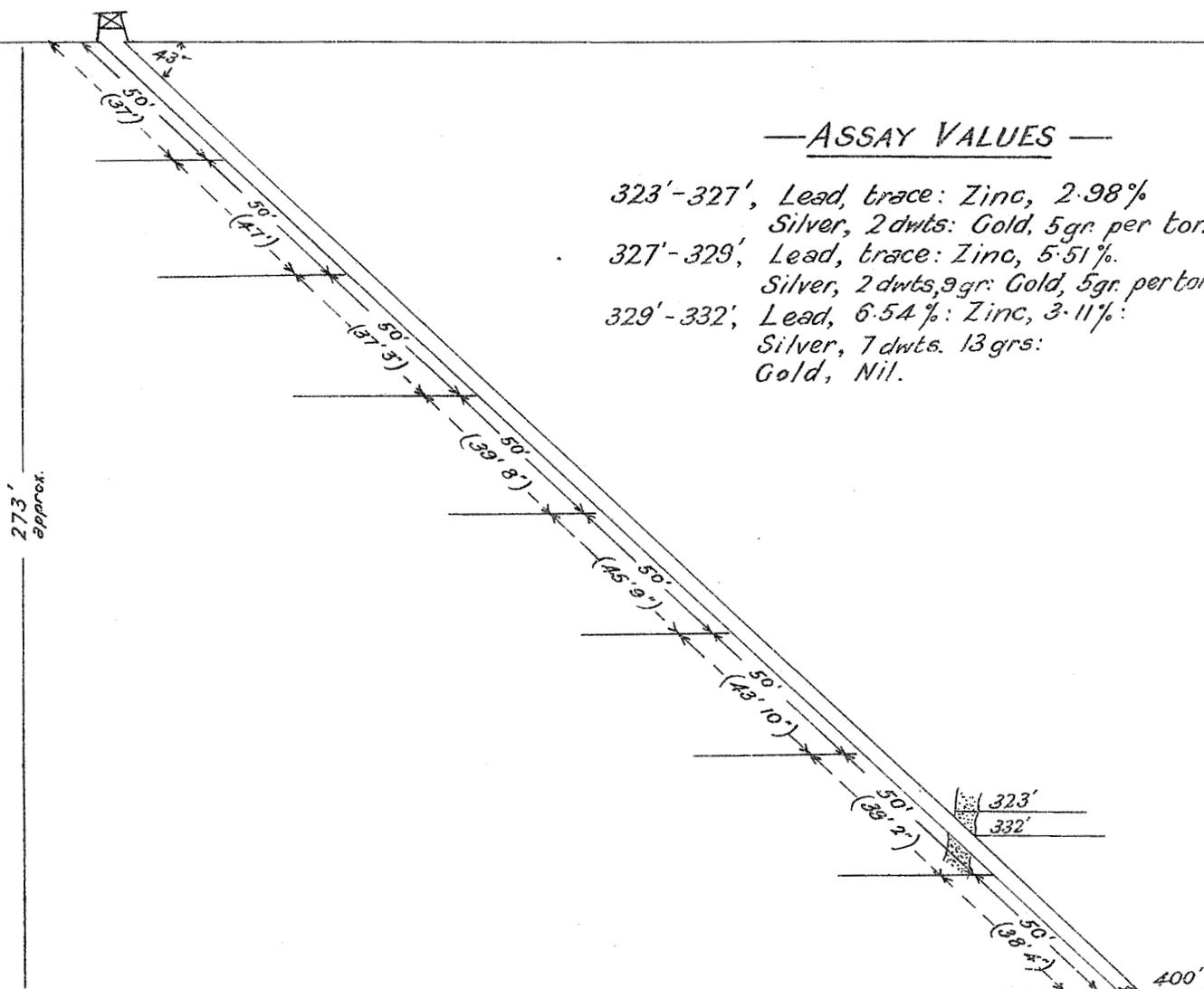
Figures in brackets indicate the length of core recovered from the corresponding section of boring.
