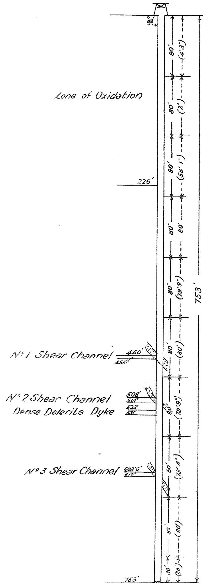
Figures in brackets indicate the length of core recovered from the corresponding section of boring.
