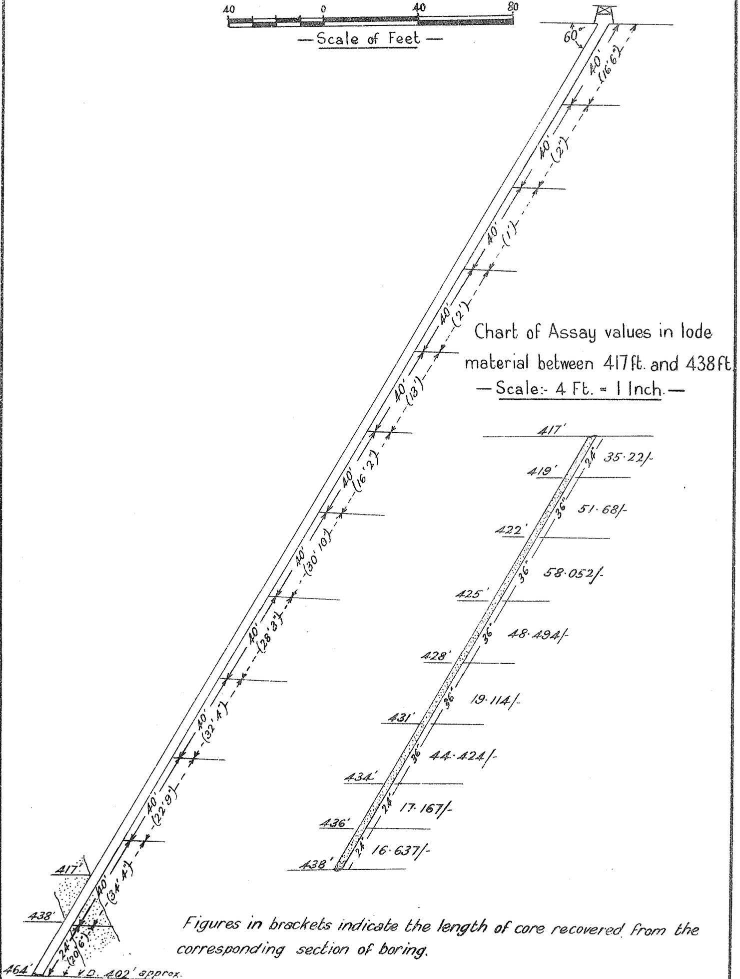
Figures in brackets indicate the length of core recovered from the corresponding section of boring.
