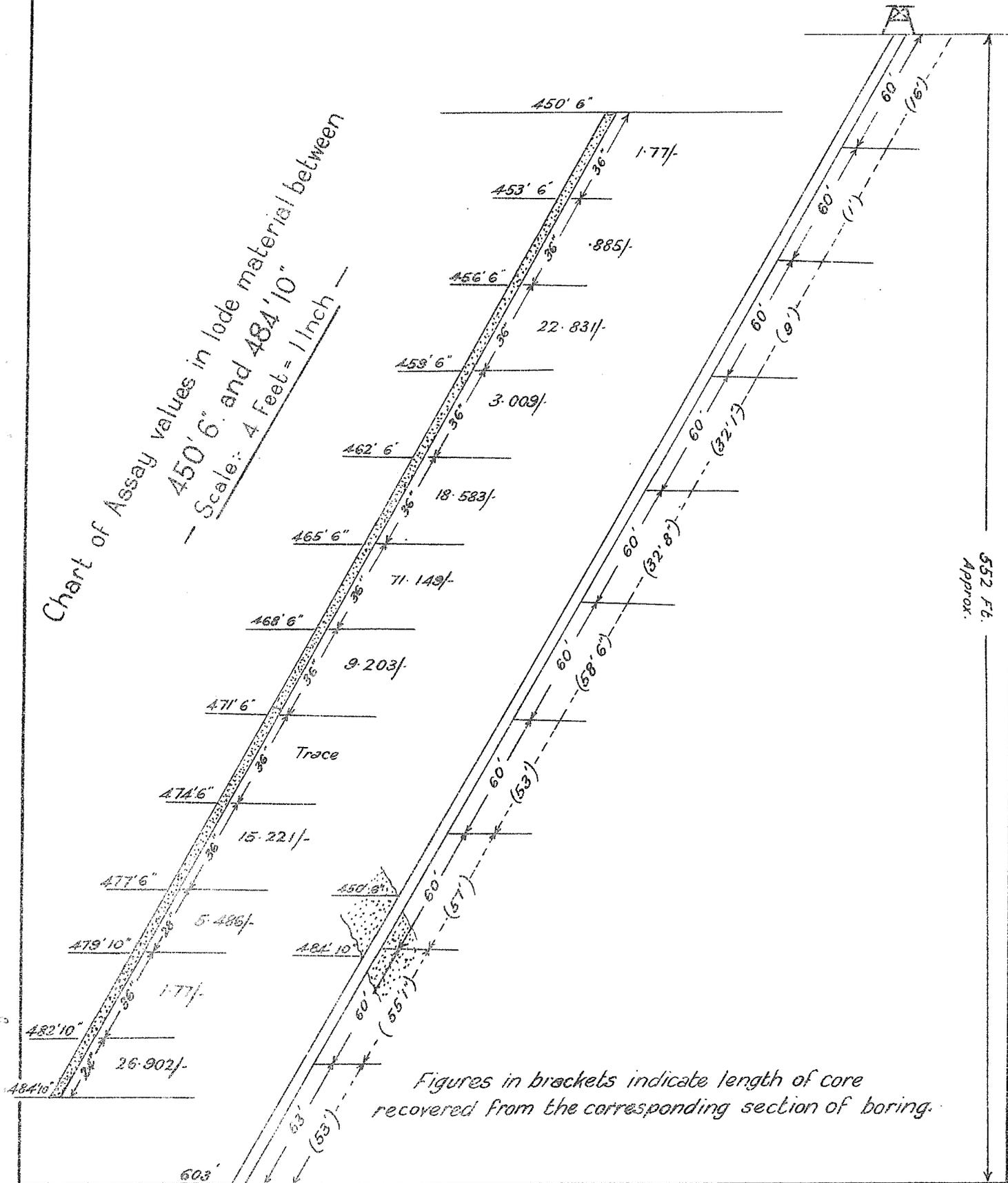
Figures in brackets indicate length of core recovered from the corresponding section of boring.
