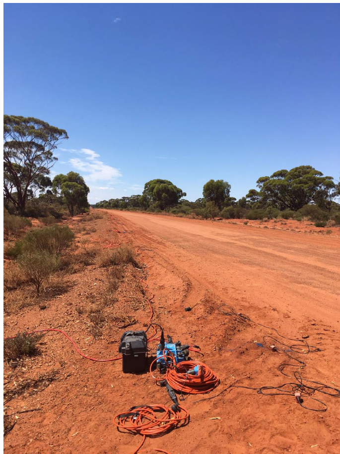
Figure 3. Geophone receiver group in spread along road verge
