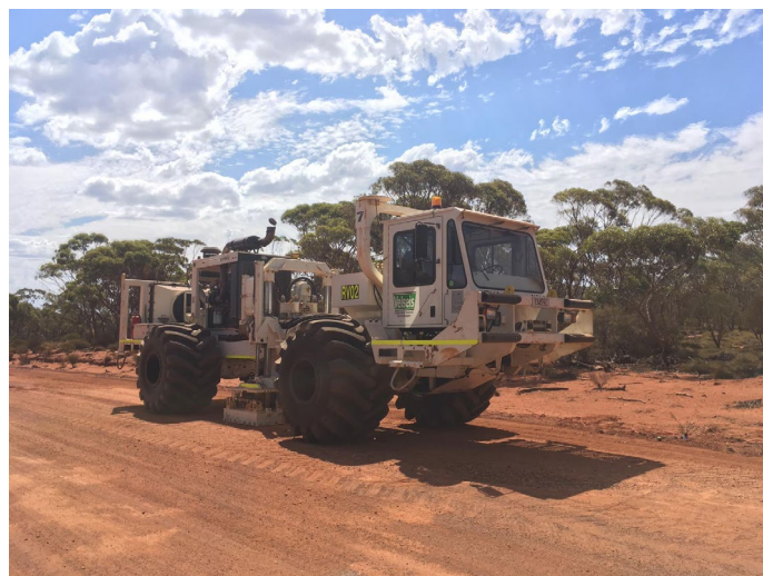
Figure 2. AHV-IV 380 Renegade Vibroseis truck on line during survey
