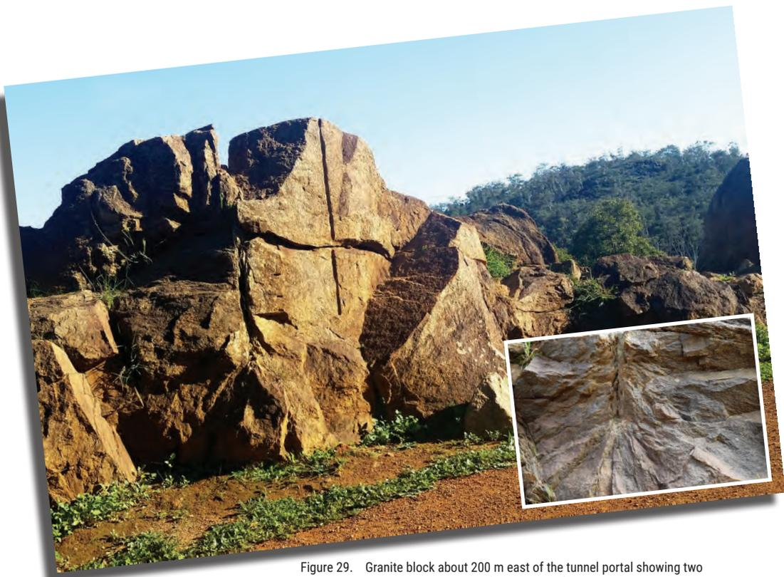
Figure 29. Granite block about 200 m east of the tunnel portal showing two drillholes. The western (left-hand side) hole was charged with explosive. The radial fractures at the bottom (inset) show where the blast occurred. The eastern hole has no star-shaped fractures and was not blasted
