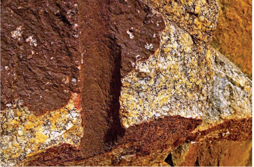
Figure 8. Dark iron oxide coating on granite surface. Note the drillhole, used to hold the explosive to blast the rock apart, has the coating as well as the broken rock surface showing how quickly the surface stain can form. Fresher granite in the middle of the photo is slightly yellowish, and discoloured through the early stages of weathering
