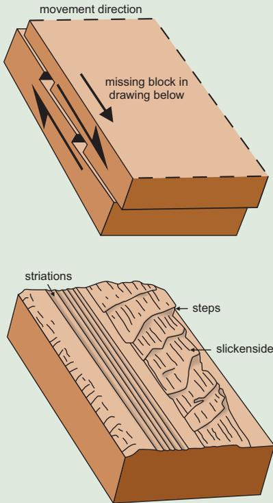
Figure 10. Block diagram showing how sliding on a fault creates a slickenside and its striations and other features
