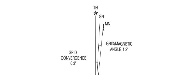
True north, grid north and magnetic north are shown diagrammatically for the centre of the map. Magnetic north is correct for 1995 and moves easterly about 0.1° in five years
