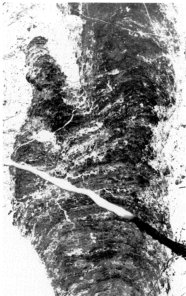
Figure 3. Part of a column of Pilbaria perplexa , showing typical niche and pocket development. Polished slab of GSWA F 46610 —5 km north-east of Paulsen Mine, WYL 29.
