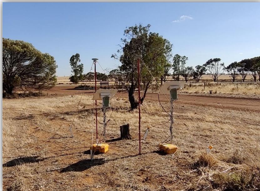
Photo 5 – A Leica GX1230 GNSS receiver set up over base 1260 with a redundant base set up nearby
