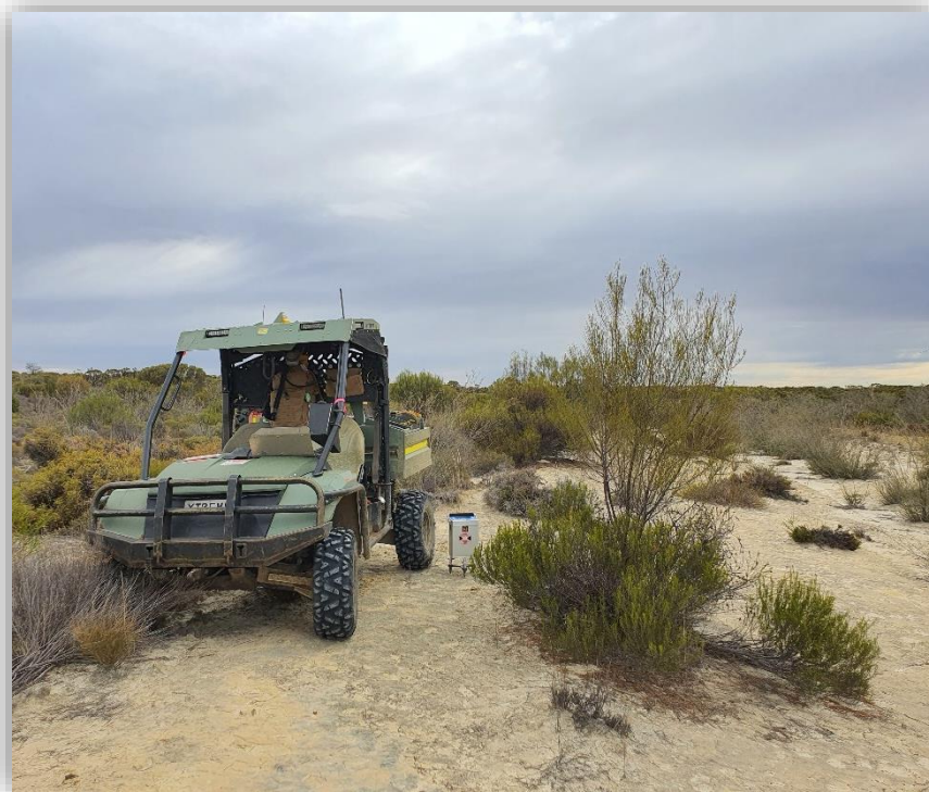
Photo 3 – DATV with CG5 gravity meter performing a gravity observation
