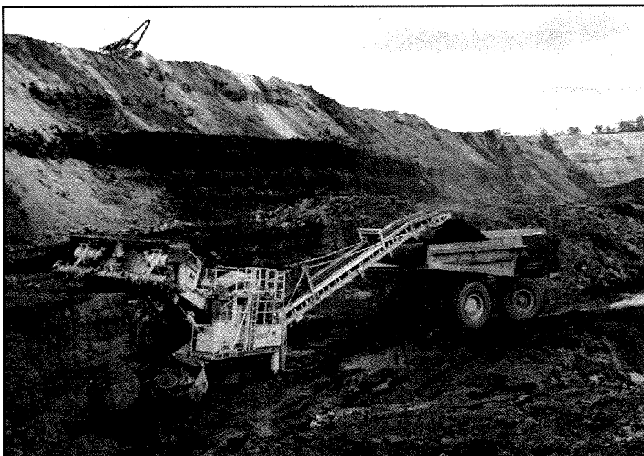
Δ A "Continuous Miner" gnaws away at a coal seam near Collie.
