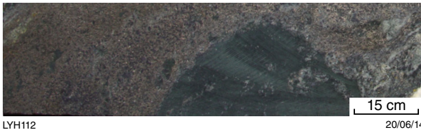
Figure 19. Semi-massive sulfides, magnetite, carbonate, and quartz interstitial to ragged areas of mafic rock (GSWA 208103 from 270.5 m in YD10-01)
