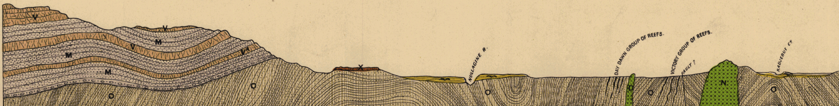
GENERALISED SECTION ACROSS THE VALLEY OF THE NULLAGINE RIVER SHEWING (a) THE NULLAGINE SERIES WITH INTERBEDDED IGNEOUS ROCKS, AND (b) THE MOSQUITO CREEK BEDS WITH INTRUSIVE IGNEOUS ROCKS.
