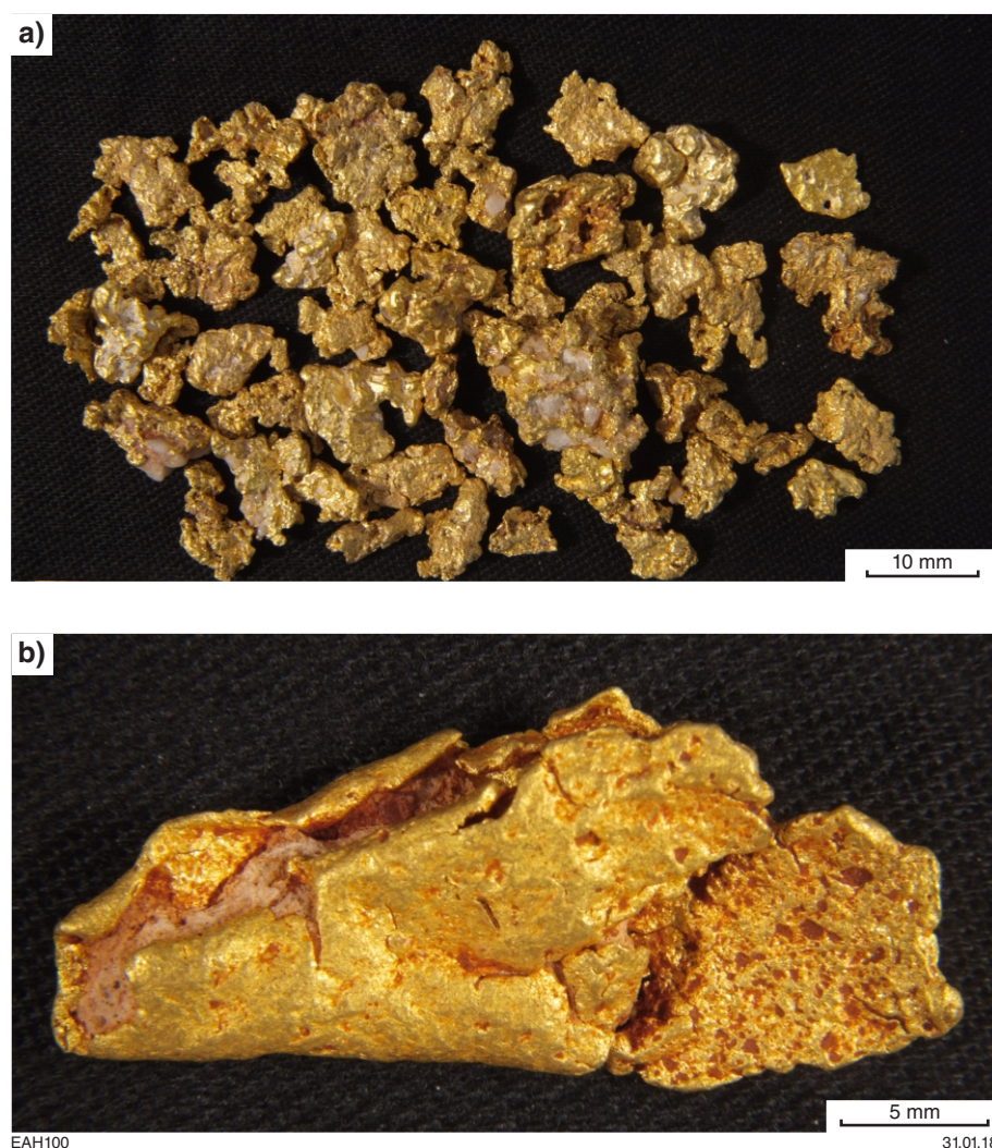
Figure 2. Morphology of gold nuggets: a) angular irregular with pitted and spongy surface, intergrowth with milky quartz; sample GSWA 201951; b) well-rounded and folded with even and smoothed pitted surface, inclusions of ferruginous clay mixture; sample GSWA 201946
