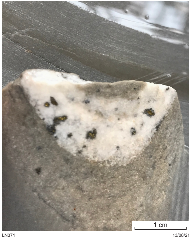
Figure 47. Visible copper mineralization in GSWA sample 226264 at 2661.13 m; multi-element analysis yielded 1240 ppm Cu
