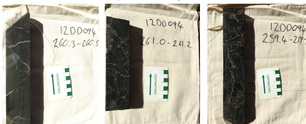
Figure 20: Volcanic core samples of 12942603, 12941610, and 12942594 that show stockwork veining of quartz-carbonate veins.
