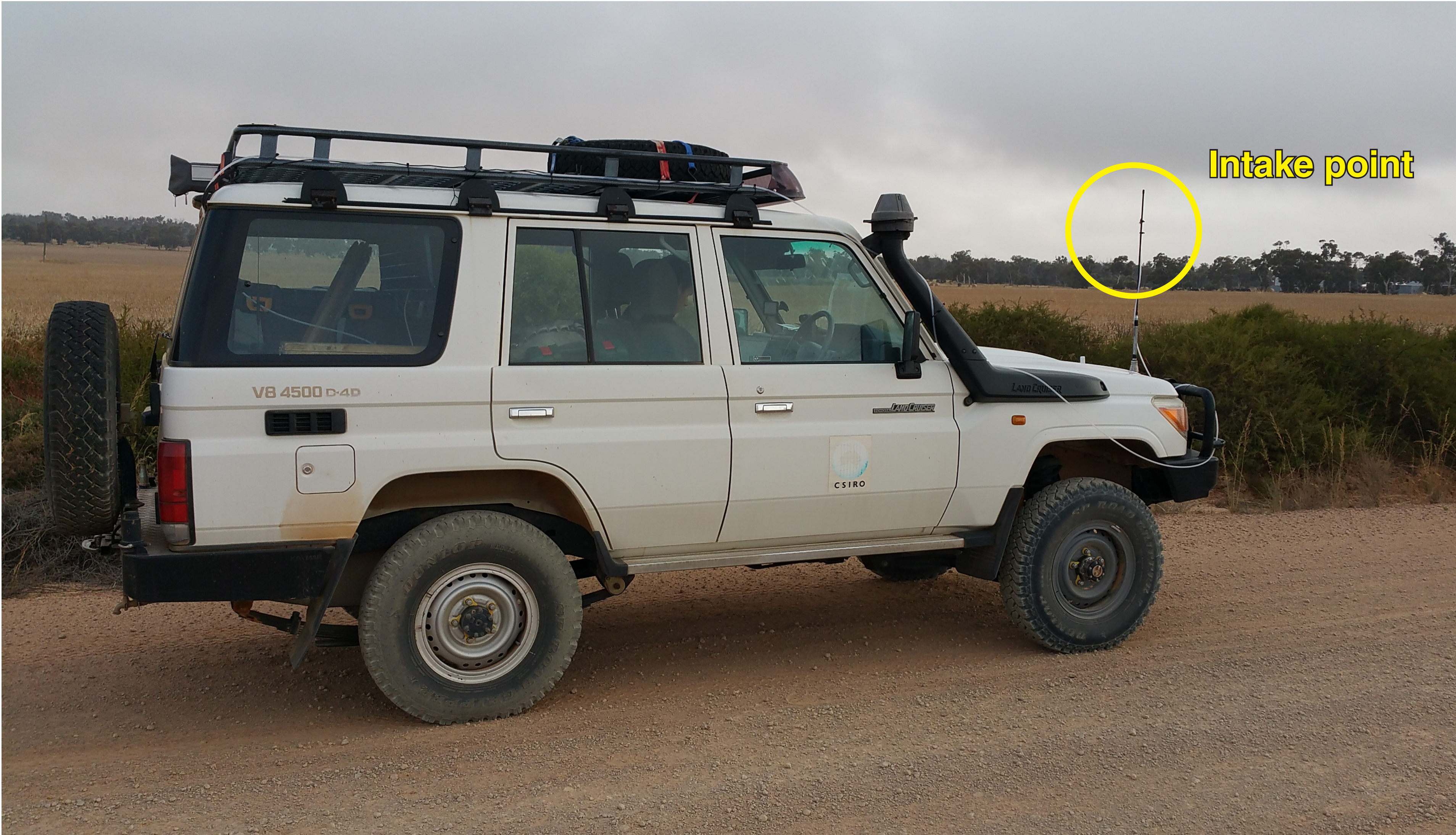
Vehicle set up for mobile survey showing the intake point attached to the antenna of the vehicle.
