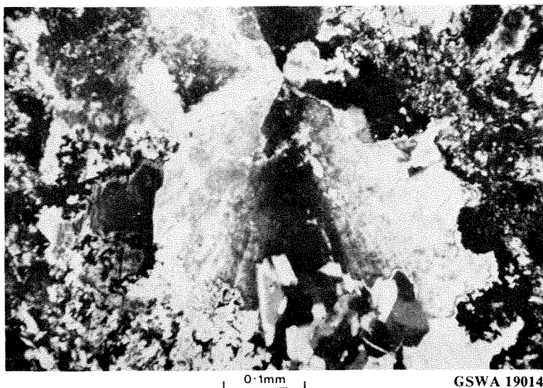
Figure 16. Photomicrograph of prehnite within the Honeyeater Basalt, 10 km north of Soanesville. Crossed polars. GSWA 49383 .
