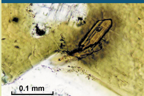
Baddeleyite crystals showing radiation halo in dolerite
