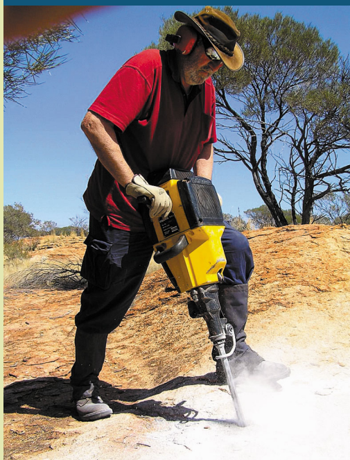
Peter Boner drilling to obtain unweathered samples
