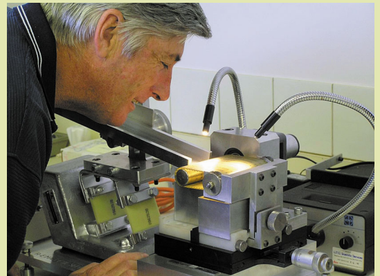
Lab manager John Williams with rare-earth magnetic separator
