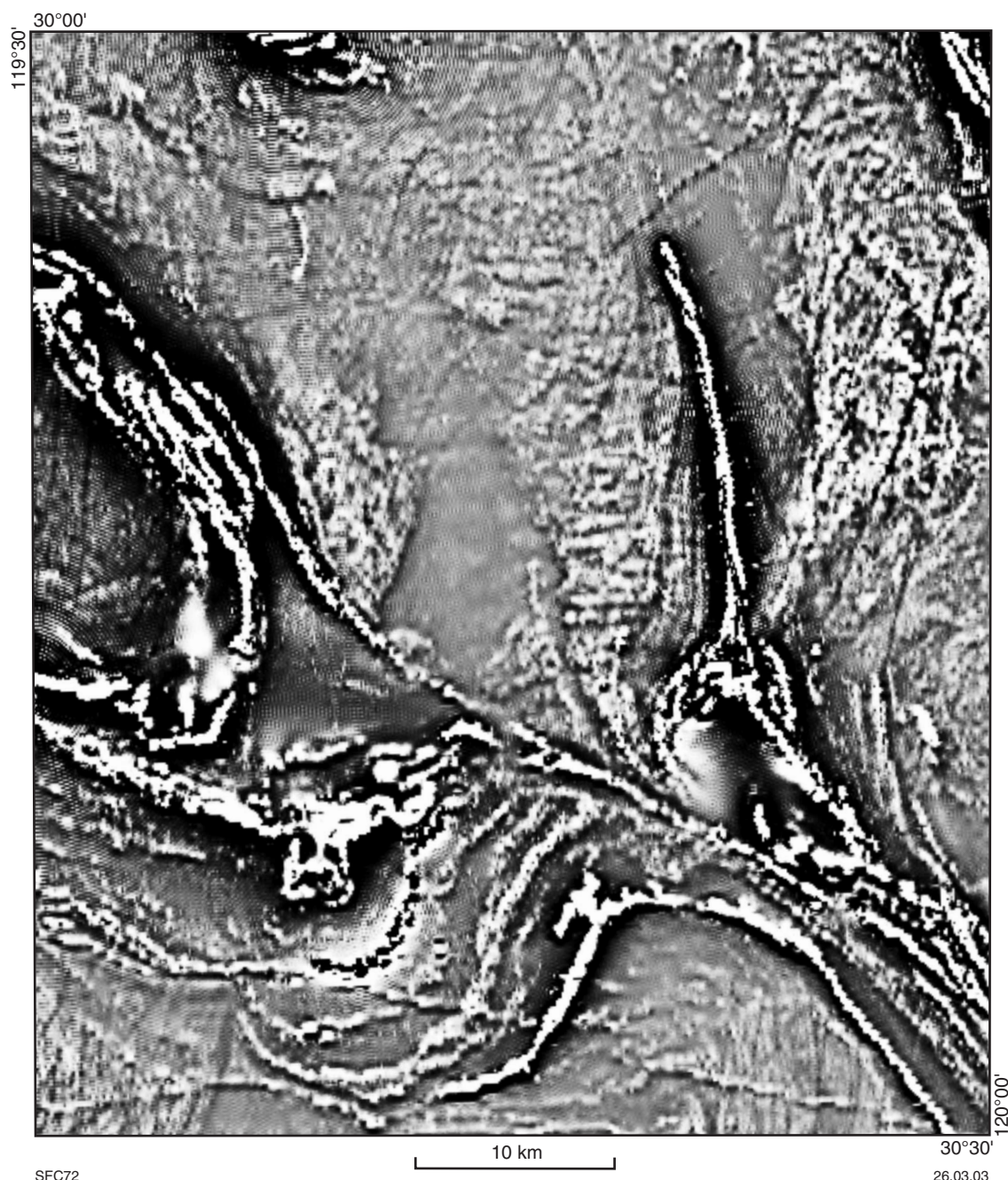
Figure 5. First vertical derivative aeromagnetic image of BUNGALBIN (based on 400m line-spaced data)
