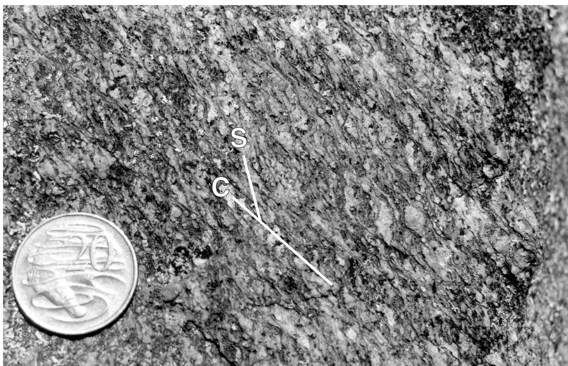
Figure 12. S-C fabrics in strongly foliated monzogranite (MGA 747600E 6666700N), showing sinistral shear sense in the Mount Dimer Shear Zone. Asymmetric feldspar porphyroclasts also indicate sinistral shear sense
