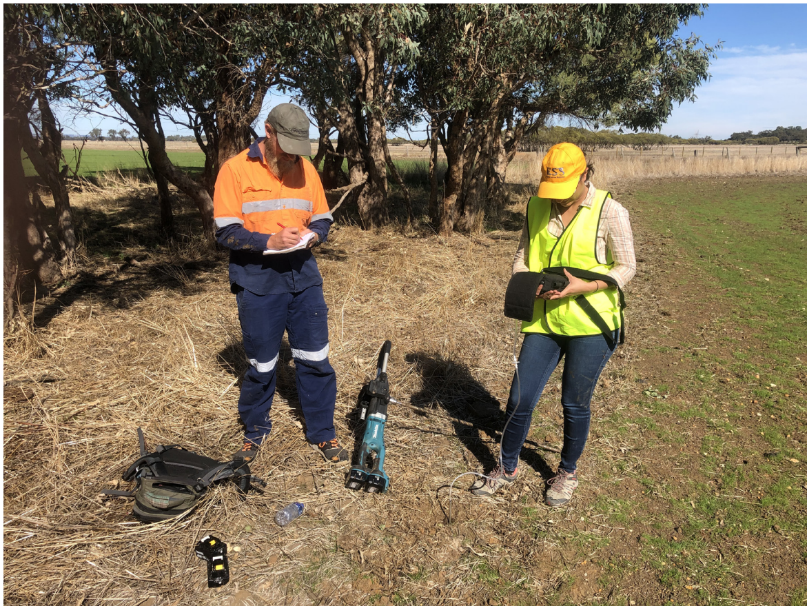
Figure 3. Taking soil gas measurements near Harvey 2 wellsite to detect natural hydrogen and other gases
