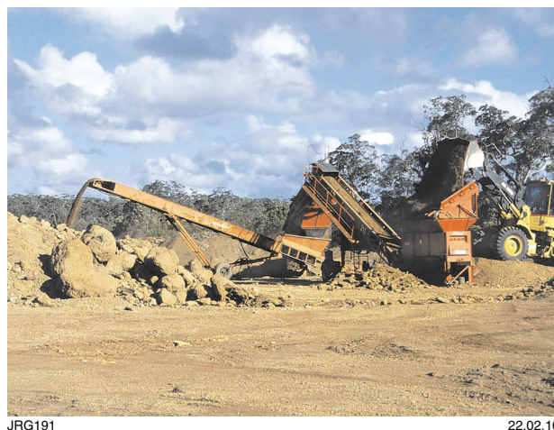
Figure 76. Screening and grading lateritic gravel
