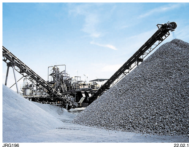
Figure 72. Crushing and grading hard rock aggregate
