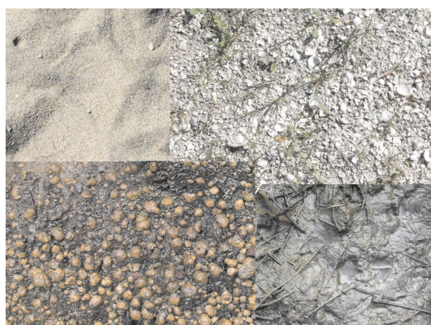
Figure 51. A variety of surface material textures: Top left: sand Top right: shelly limestone Bottom left: lateritic gravel Bottom right: clay
