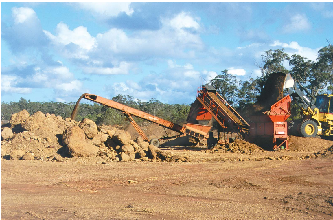
Figure 8. Active gravel pit in ferruginous lateritic duricrust (CoRf) within state forest south of Rosa Brook Road (MGA 326015E 6238385N). The pit is operating in about 2 m of gravel
