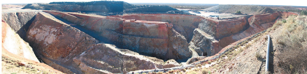
Figure 47. Panorama of the Lancefield deposit highlighting the convex nature of the pit and the Lancefield shear zone
