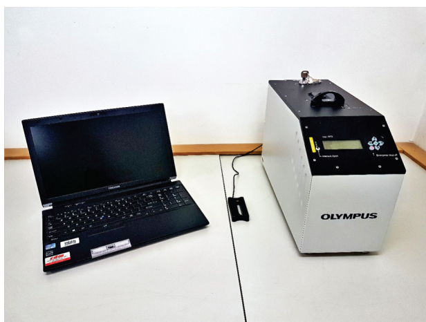
Figure 6. The GSWA benchtop XRD with external shaker and WiFi-connected laptop
