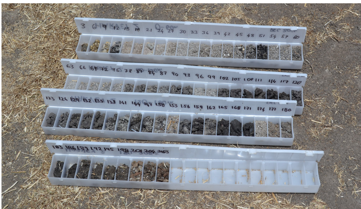
Figure 40: DMP Harvey 2: drill chip trays from the openhole rotary drilling of the superficial sediments and Leederville Formation.
