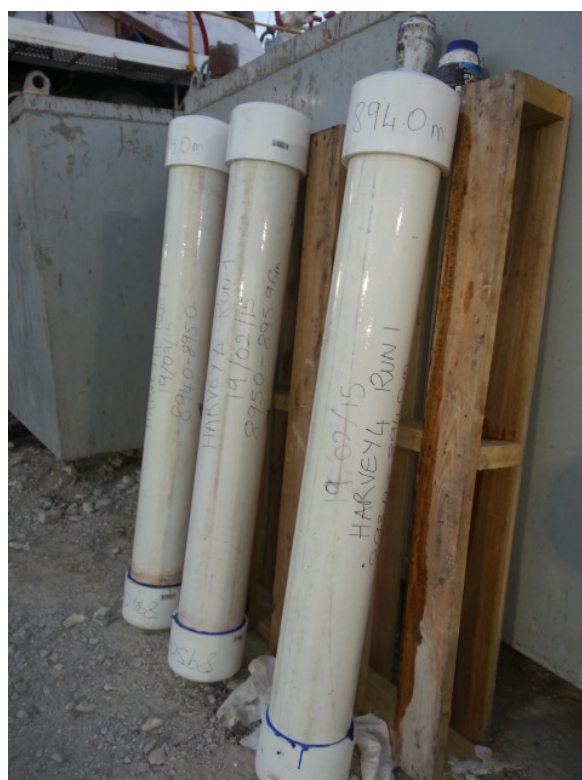
Figure 39: DMP Harvey 4: mudstone-rich facies (paleosols) preserved in mineral oil filled PVC tubing, at the drill site on 19 February 2015, prior to transportation to CoreLab's premises in Kewdale.
