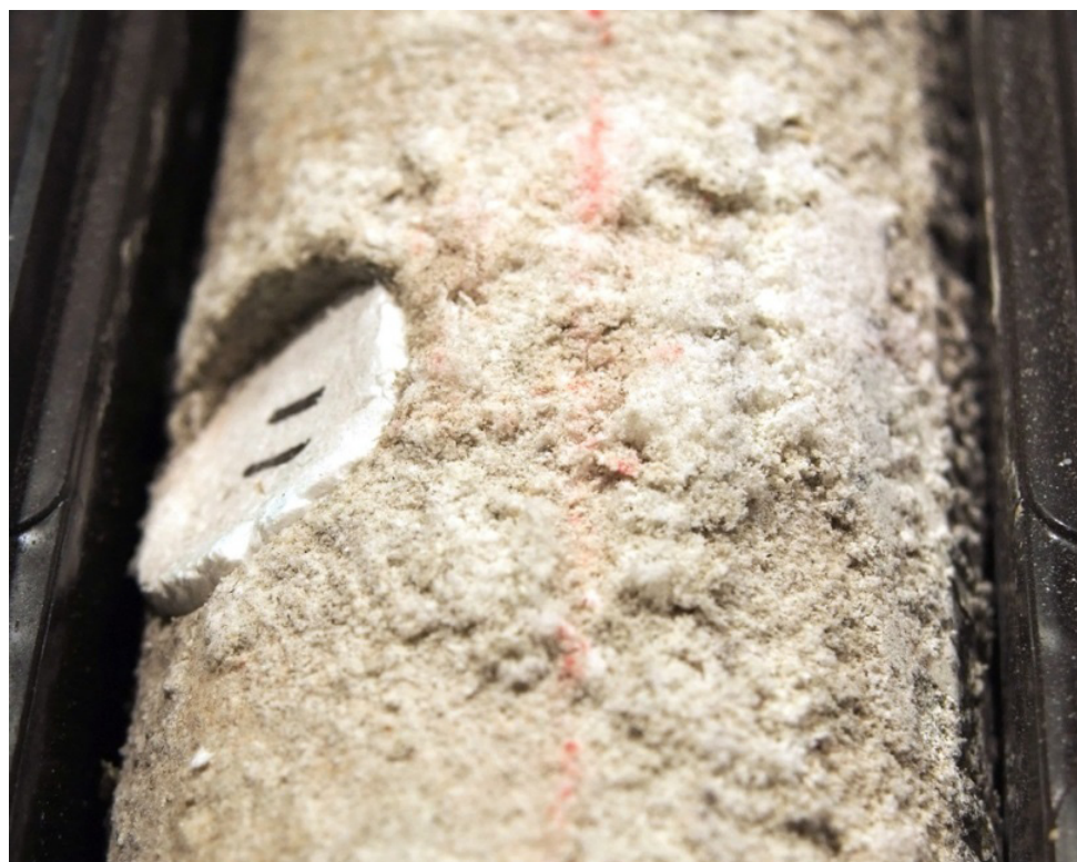
Figure 53: DMP Harvey 3: a close-up of the Wonnerup Member core shown in Figure 52. The white crystals on the core's surface are sylvite, a potassium chloride (KCl) evaporitic salt; the drilling fluid invaded the formation and subsequently evaporated at the core's surface.
