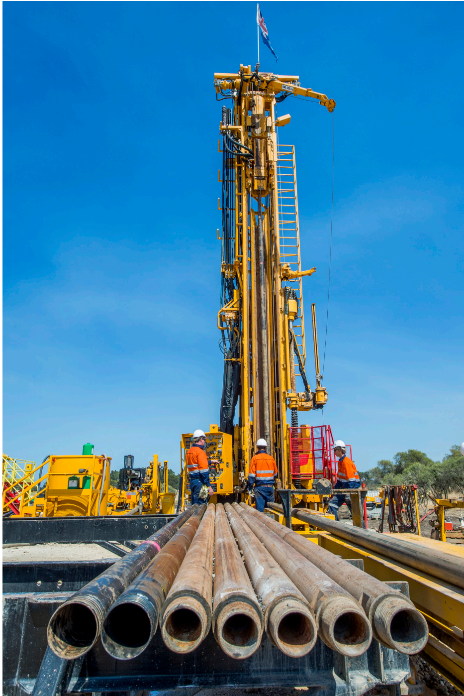
Figure 17: DDH1 Drilling Pty Ltd's Evolution 3000 rig (Rig 16) drilling DMP Harvey 3 (Henderson Photographics for DMP).
