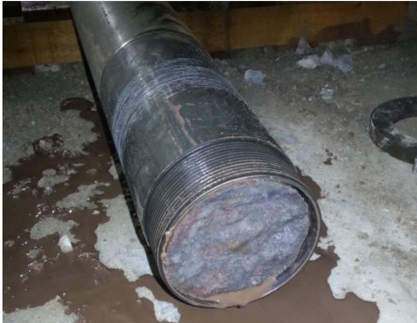
Figure 37: DMP Harvey 4: SQ-sized (120mm diameter) inner core barrel containing freshly cut core retrieved during interval coring of the Yalgorup Member. The core is contained within a plastic sleeve within the inner core barrel.
