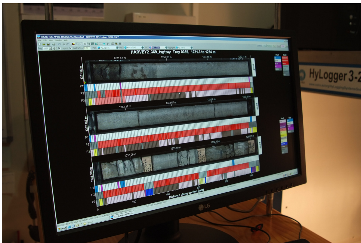
Figure 46: HyLogger screen image for DMP Harvey 2 core from 1231.3 to 1234.0m depth. Images of each one-metre length of core and the shortwave infrared (red and salmon pink) and thermal infrared (pink and brown) spectrometer images can be seen, providing the mineralogical composition. In this screen image the dominant minerals are kaolinite and quartz, from the interbedded sandstones and mudstones at the base of the Yalgorup Member.
