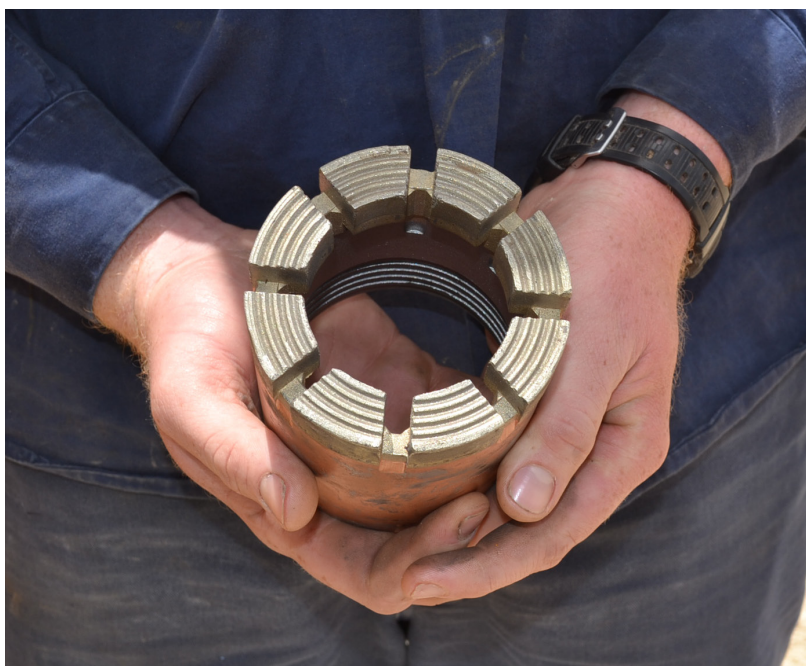
Figure 22: HQ3-sized diamond-impregnated core bit used in the drilling of the HQ-sized Wonnerup Member sections of DMP Harvey 2 and 3, December 2014.
