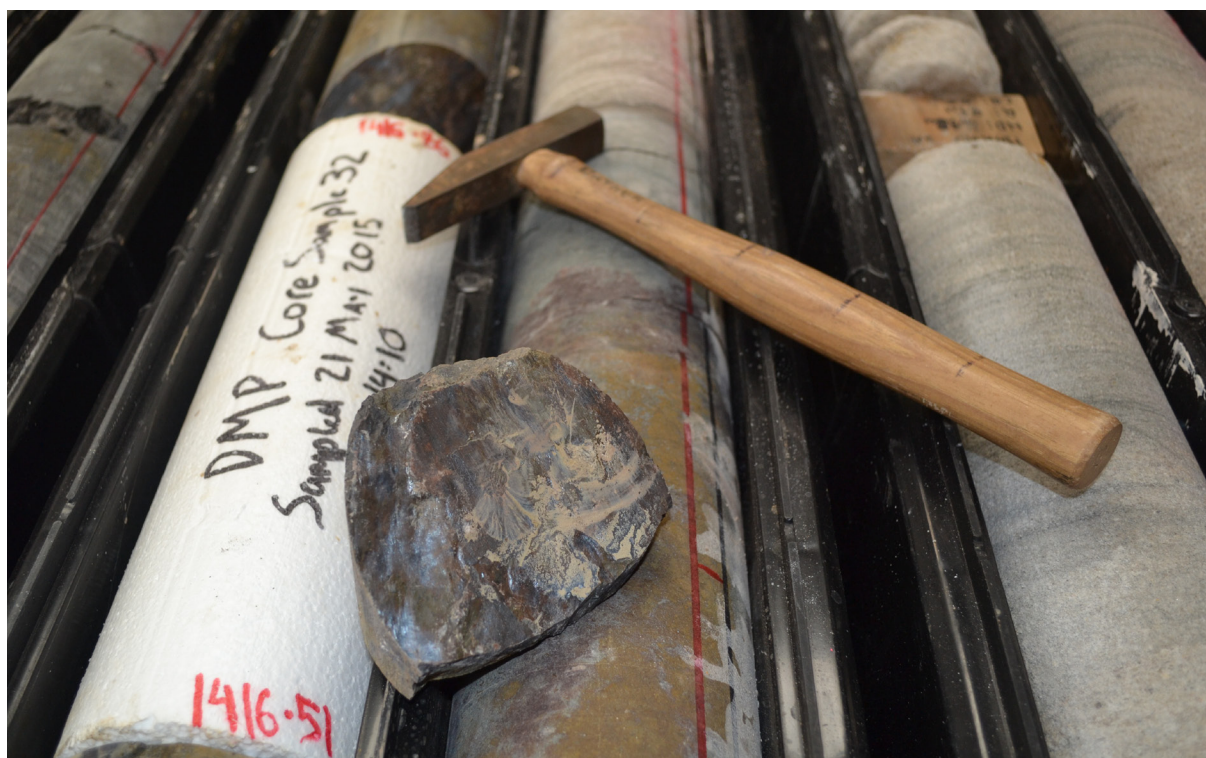
Figure 36: DMP Harvey 3: slickensides (shiny surface) within the paleosols in core from the base of the Yalgorup Member, above the boundary between the Wonnerup and Yalgorup Members.
