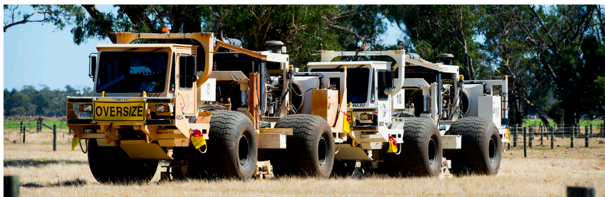
Figure 5: Vibroseis trucks working in tandem during the Harvey Waroona 3D seismic survey (Geokinetics Pty Ltd, April 2014).
