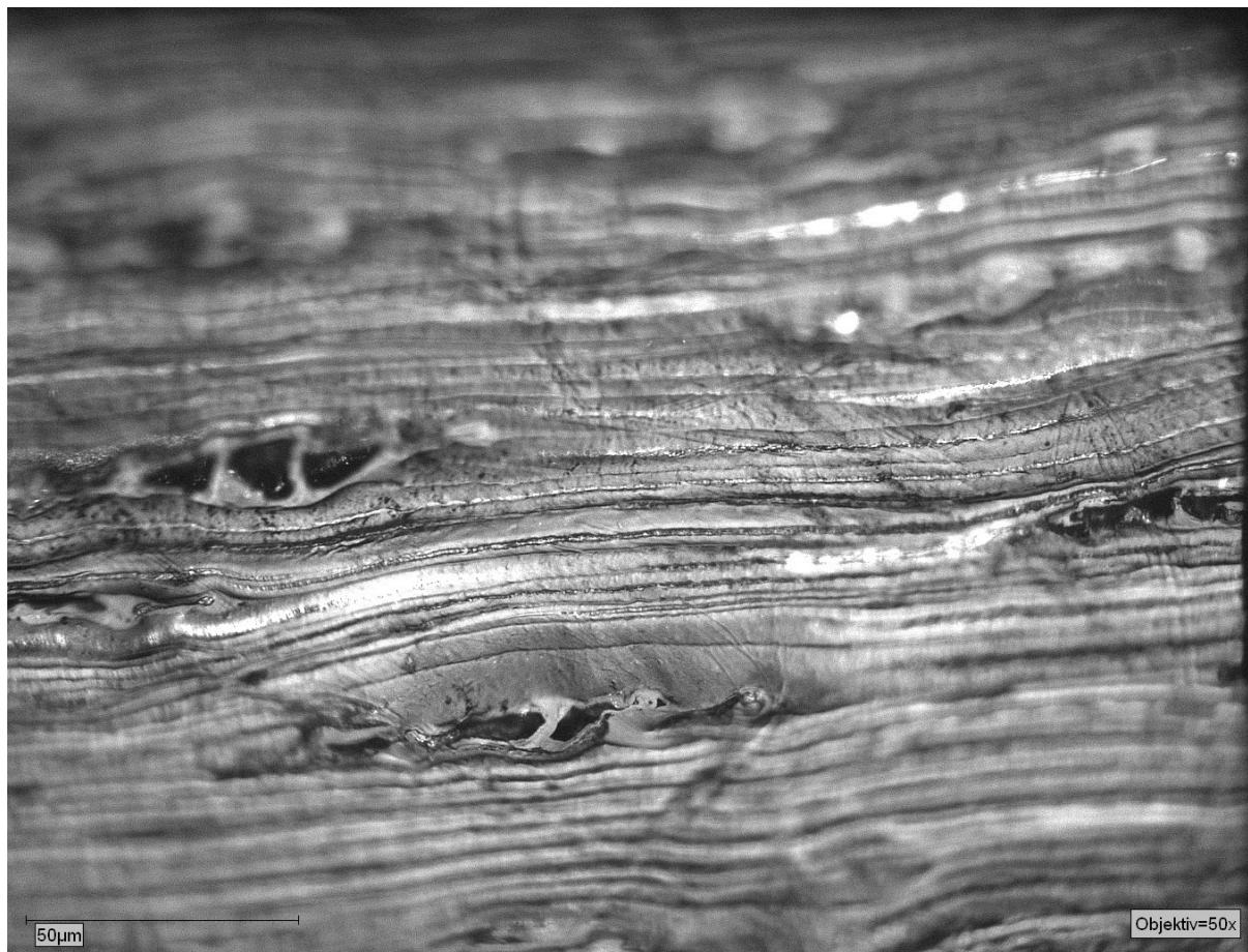
Figure 86: Mounted sample from 841.66m depth in DMP Harvey 3 in reflected white light (magnification 50x), showing telinite with unaltered cellulose.
