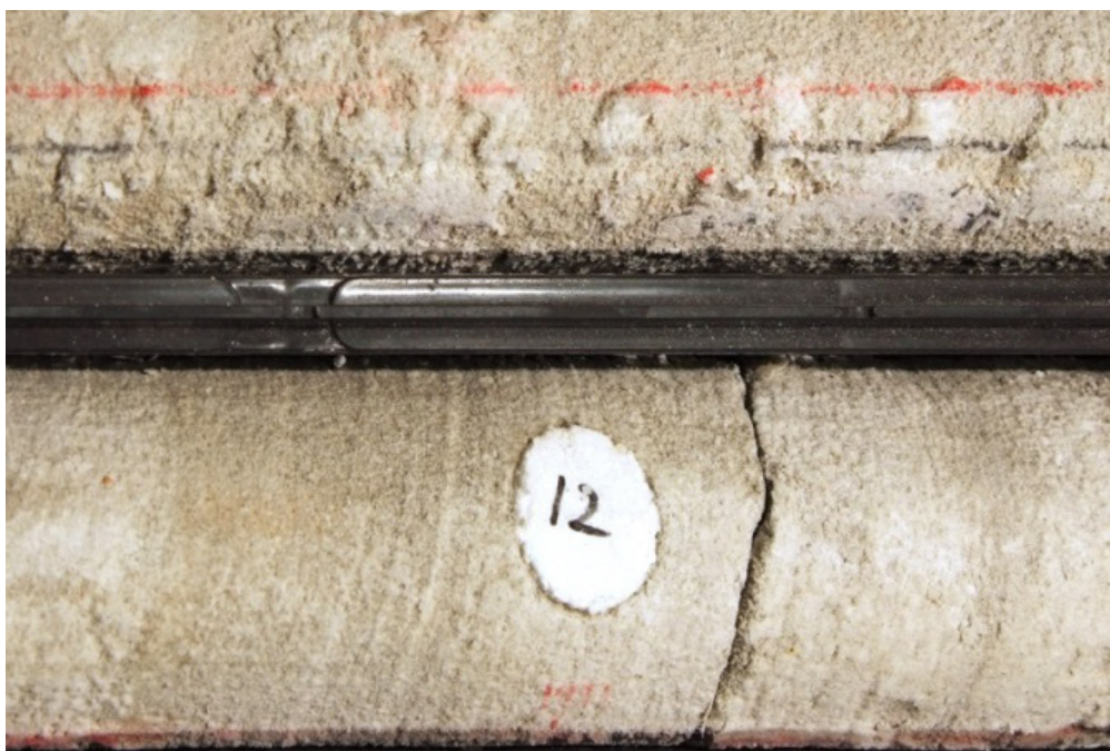
Figure 52: DMP Harvey 3 well: SQ3-sized core from the Wonnerup Member at approximately 1500m depth, in tray 406, showing the locations of core plugs 11 and 12.
