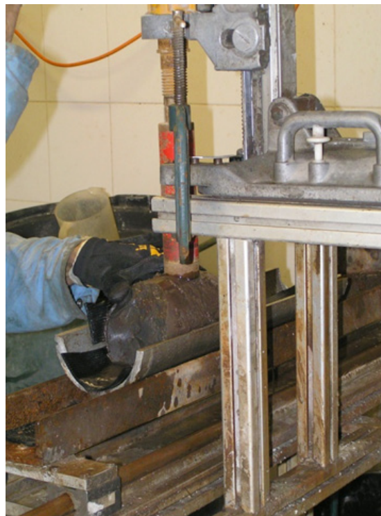
Figure 43: CoreLab's technician cutting a horizontally orientated, 1.5-inch diameter plug from a mineral oil-preserved interpreted paleosol at 697m depth in DMP Harvey 3.
