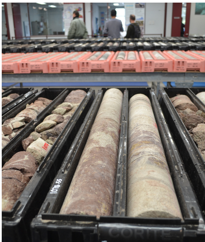
Figure 35: DMP Harvey 3: SQ3-sized core (102mm) between 1078.55 and 1080.40m, in core tray 224. These are considered to be paleosols within the Yalgorup Member.
