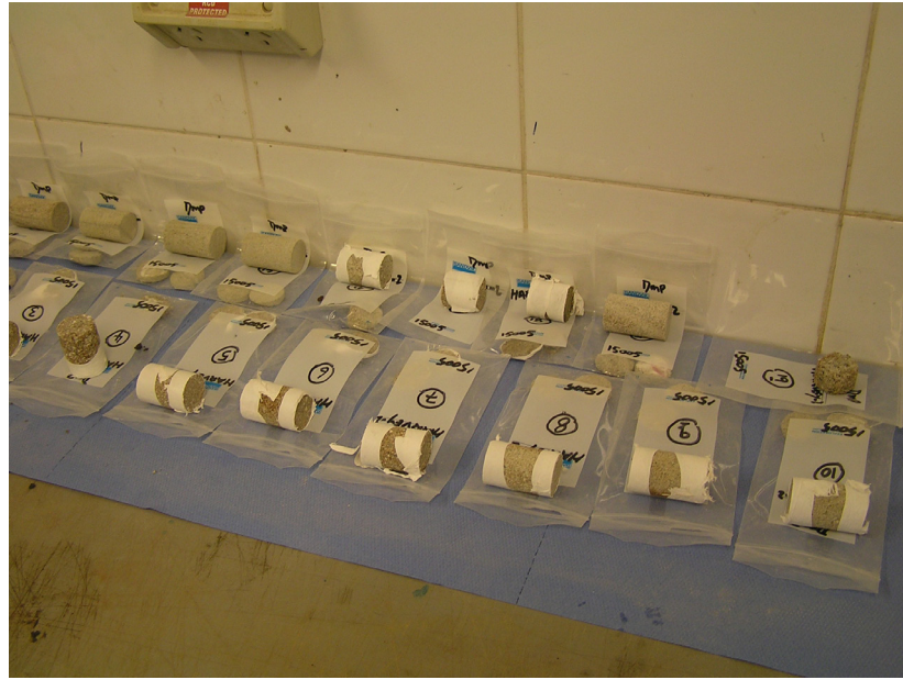
Figure 42: Cut and labelled sandstone-rich plugs cut from the Wonnerup Member in DMP Harvey 2, 3 and 4, at CoreLab's premises, Kewdale.
