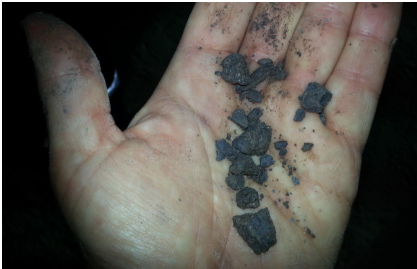
Figure 38: DMP Harvey 4: grey, cemented, brittle mudstone from an interpreted paleosol in the Yalgorup Member, retrieved overnight during interval coring between 893.00 and 899.30m depth. The identification of the mudstones in the freshly cored sample indicated that DMIRS' targeted coring run had been successful.
