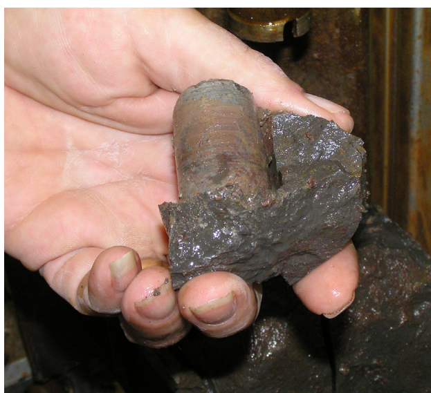
Figure 44: Cutting plug samples from core preserved in mineral oil at CoreLab's premises in August 2015. The photograph shows red iron staining of a core sample taken from paleosol mudstones within the Yalgorup Member of DMP Harvey 3.
