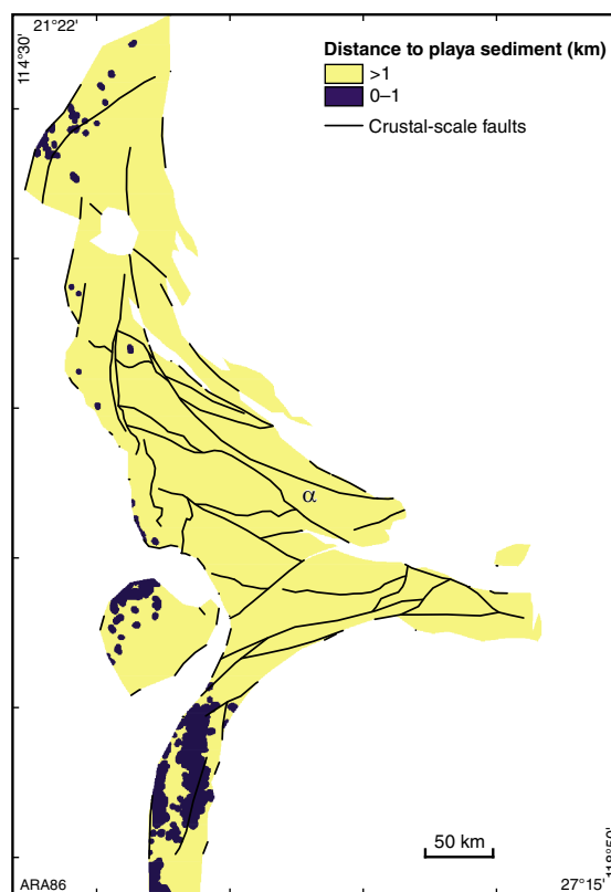
Figure 2.50. Predictor map for surficial uranium physical trap: proximity to playa sediments map. Greek letters correspond to the surficial uranium prospective zone (Fig. 25).
