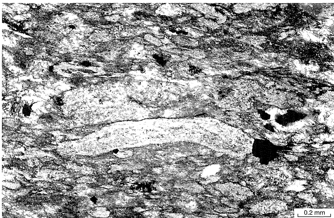
Figure 8. Photomicrograph showing pyroclastic texture (note relict shards in centre) in a mafic schist of the Narracoota Formation. GSWA 120367, plane-polarized light
