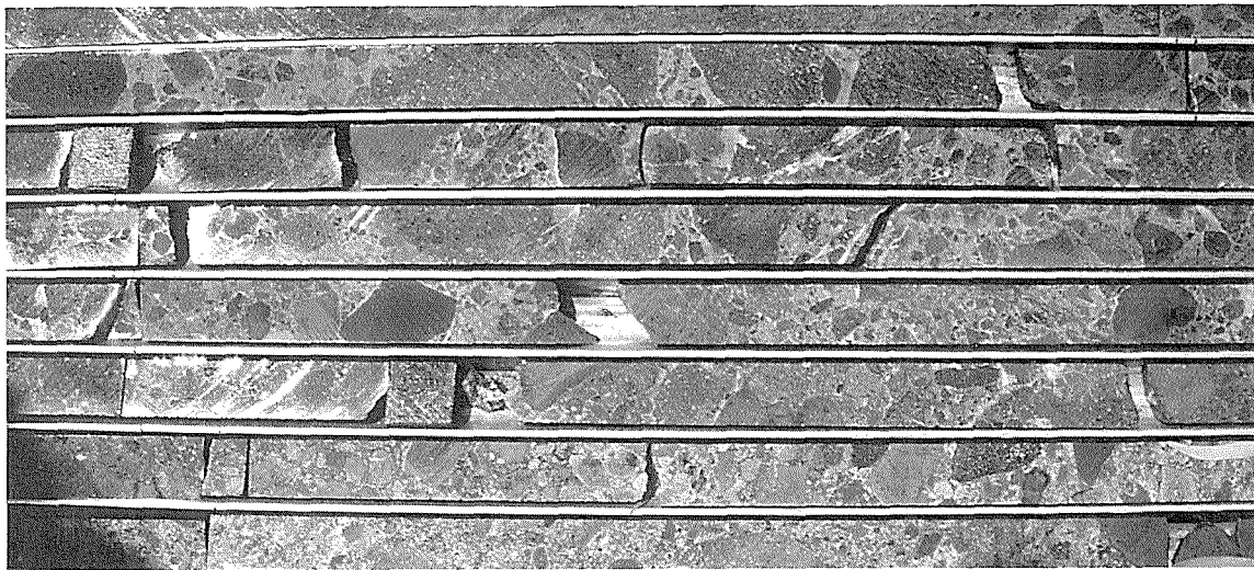
Figure 10. Volcanic breccia intersected in diamond drillhole BD1. Clasts are predominantly of basaltic rocks, and the matrix exhibits albitic alteration
