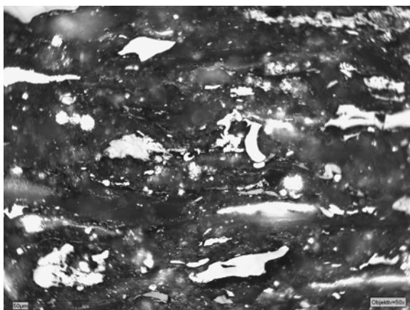
E4511G Weak fluorescing sporinite in argillaceous siltstone, reflected white light, X50
