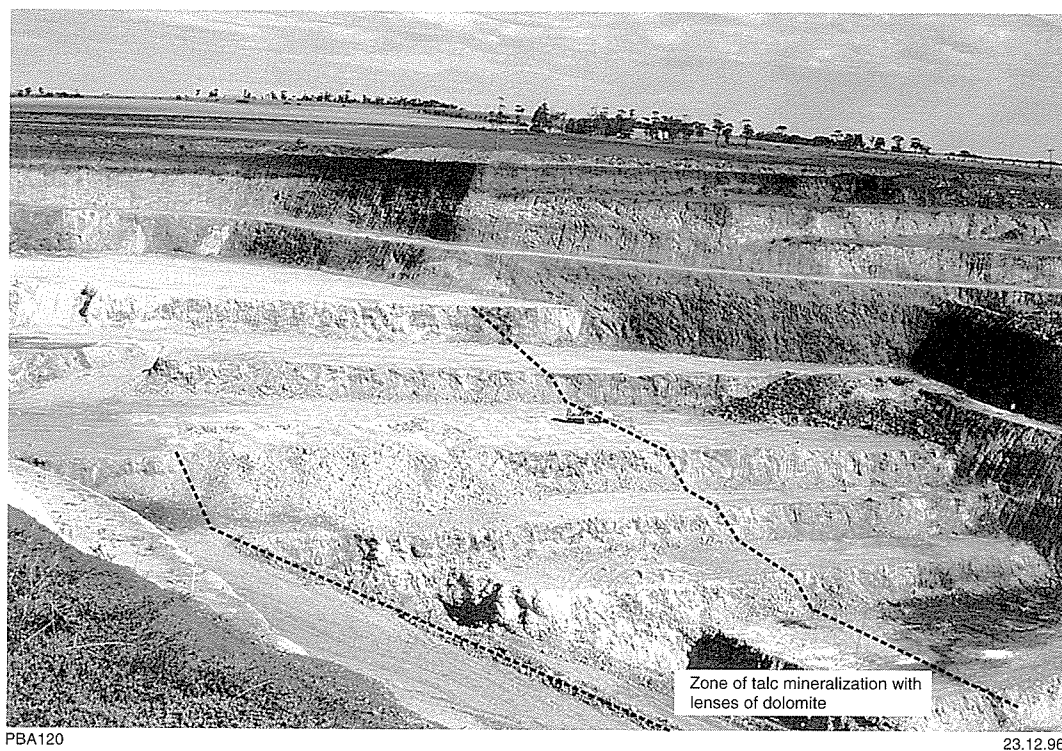
Figure 8. Photograph of openpit D at Three Springs talc mine showing zone of talc mineralization with lenses of dolomite
