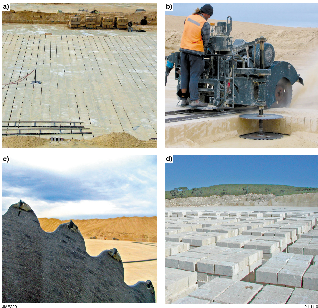
Figure 3. Extractive process for Tamala Limestone building blocks: a) the level limestone floor is cut with a series of parallel saw cuts to produce blocks in a variety of standard sizes; b) rail-mounted, multi-blade quarry saw cutting standard size blocks; c) quarry saw blade fitted with tungsten carbide cutting teeth; d) quarry-cut blocks packed on site for dispatch to clients (photo (d) courtesy Meteor Stone)
