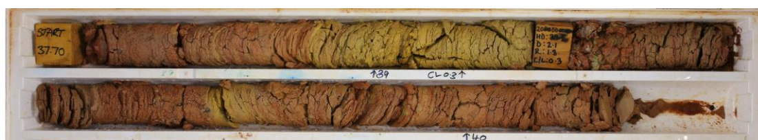
Figure 15 Oxidised Permian glacial-derived clays, 20PQDD0005A (core diameter is 7cm).
