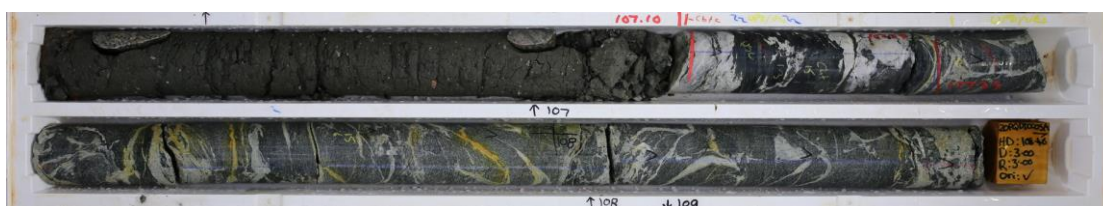
Figure 18 Fresh Archean unconformity, 20PQDD0005A (core diameter is 7cm).
