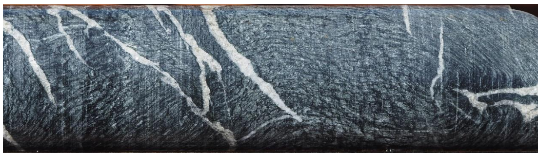
Figure 21 Strongly deformed and folded talc-carbonate altered peridotite, 20PQDD0005A (core diameter is 5cm).
