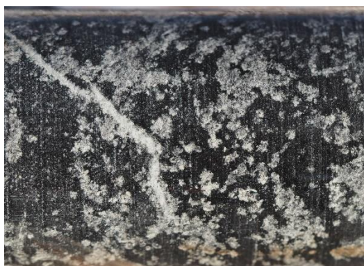
Figure 19a Talc-carbonate altered peridotite with dolomite porphyroblasts in PQDD0005A (core diameter is 5cm). Figure 19b Peridotite with potential residual serpentine PQDD0005A.
