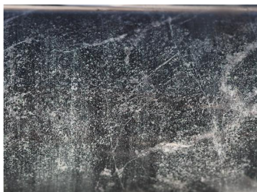
Figure 19a Talc-carbonate altered peridotite with dolomite porphyroblasts in PQDD0005A (core diameter is 5cm). Figure 19b Peridotite with potential residual serpentine PQDD0005A.
