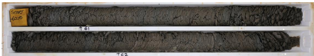
Figure 16 Reduced Permian glacial-derived laminated silts, 20PQDD0005A (core diameter is 7cm).
