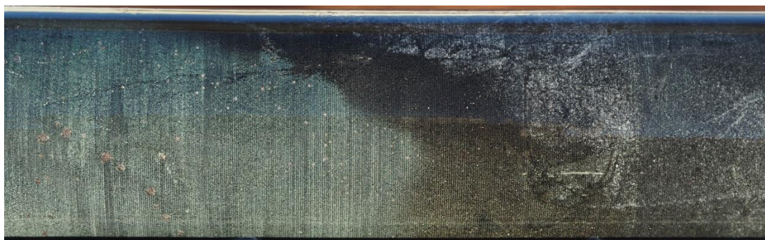
Figure 20 Intrusion (lamprophyre?) within ultramafic with biotite-chlorite-magnetite alteration, 20PQDD0005A (core diameter is 5cm).
