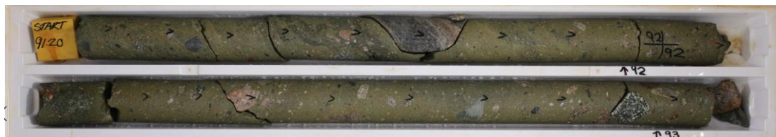
Figure 17 Indurated Permian glacial diamictite, 20PQDD0005A (core diameter is 7cm).
