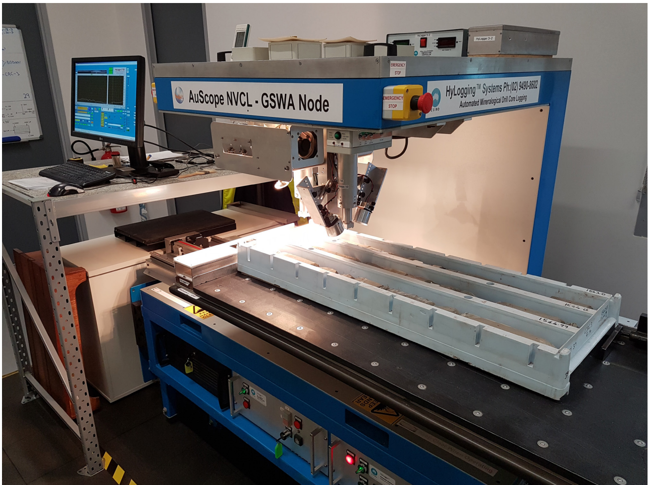
Figure 13. The HyLogger spectral scanner
