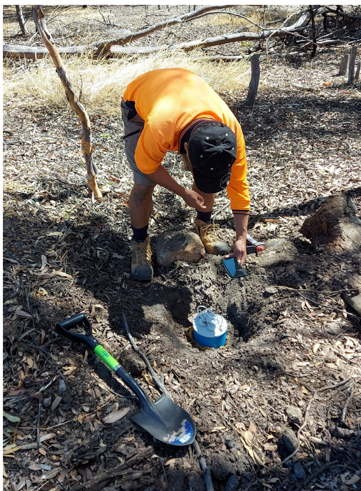
Figure 13. Installation of a SmartSolo seismometer at Arthur River aftershock monitoring site SWNNB at Warup
