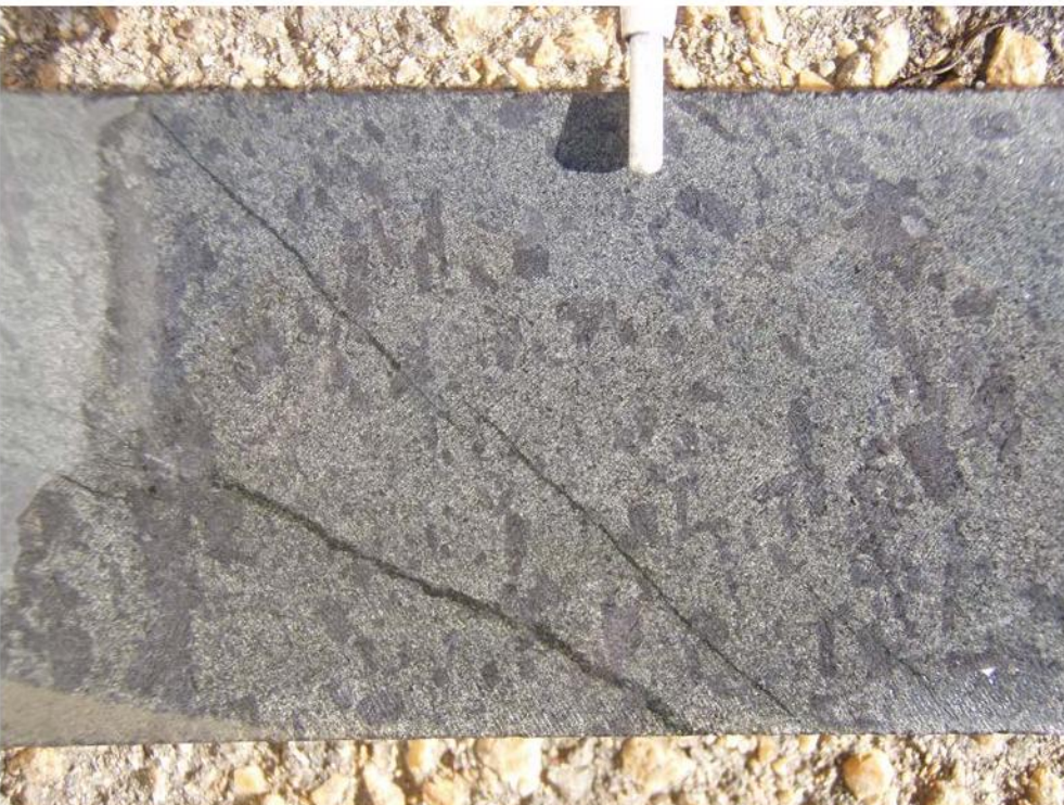
Figure 4: Typical peridotite at 206.5 metres showing flow-alignment of blocky plagioclase crystals in a finer-grained ground mass of olivine and minor clinopyroxene.
