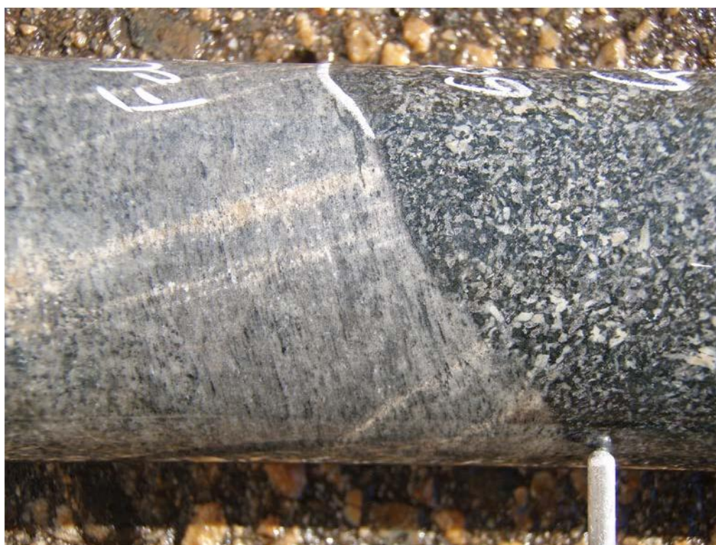
Figure 6: Sharp intrusive contact preserved between felsic meta-volcanic (left) and meta-gabbro (right) at 602.9 metres. Note truncation of quartz veins in the former.
