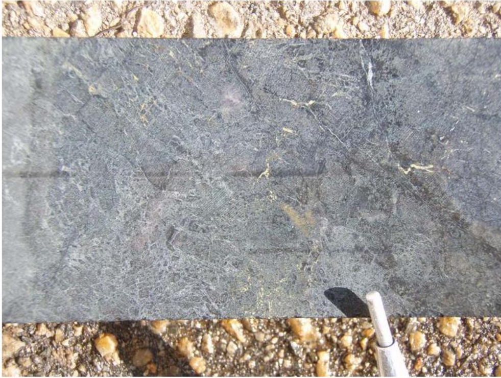
Figure 3: Coarse-grained meta-leucogabbro at 221.8 metres down hole showing blocky plagioclase habit and minor wispy chalcopyrite.
