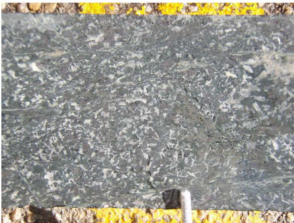
Figure 5: Typical medium-grained meta-gabbronorite at 261 metres.
