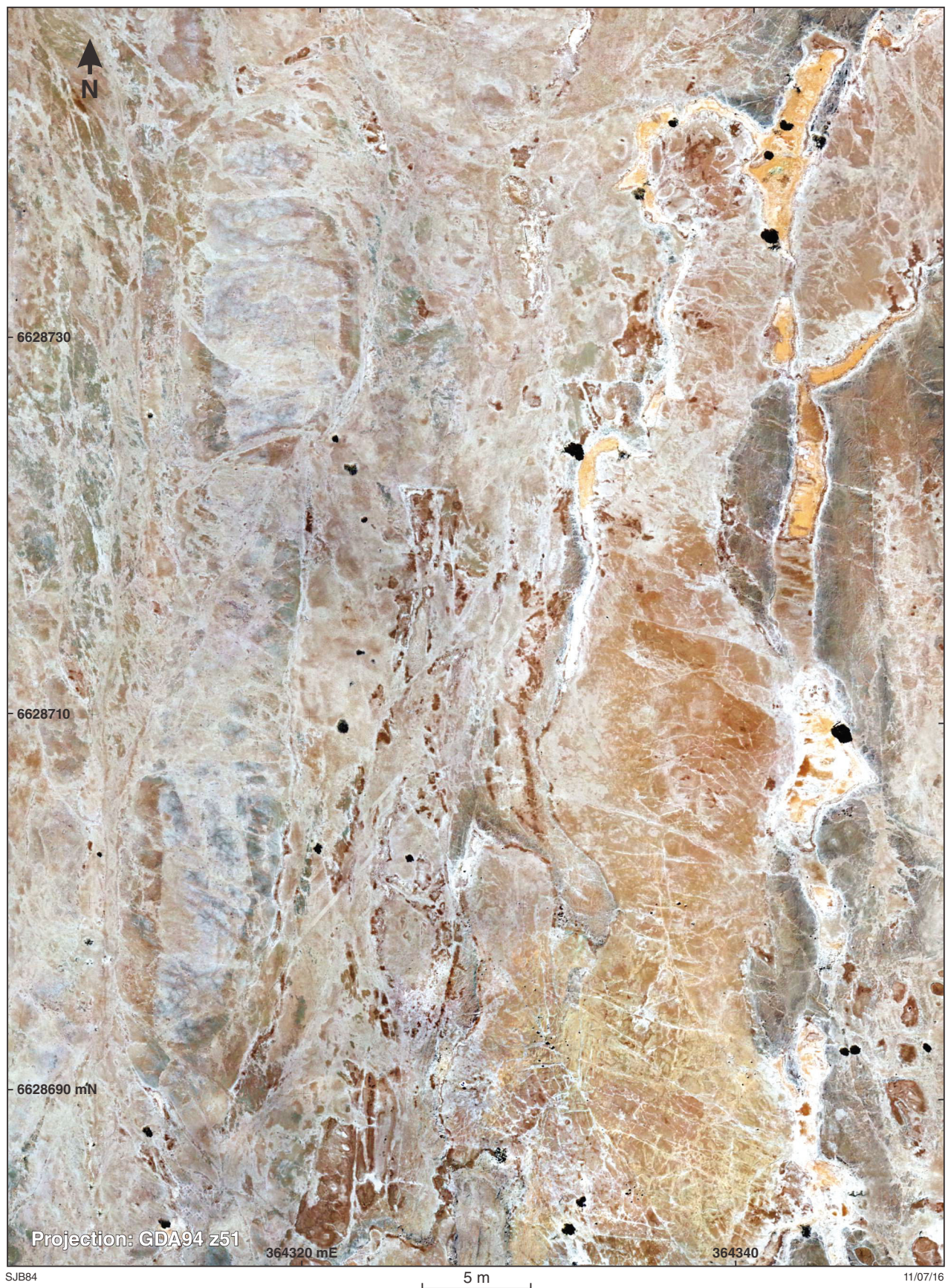
Figure 34. High-resolution orthophotos of dacite–komatiite intercalations in the Gordon Sirdar lake bed outcrops: geo-rectified photomosaics collected using drone-based photogrammetry
