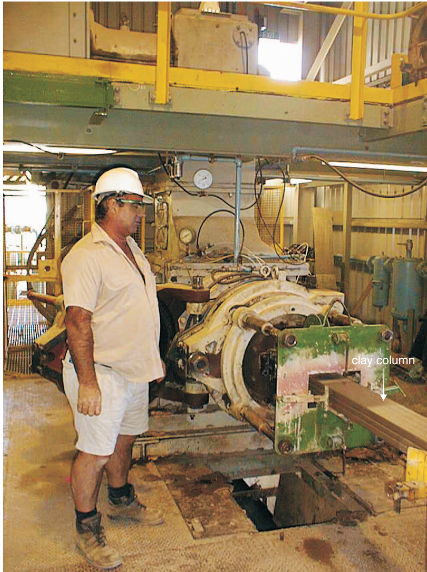
Figure 34. The extrusion of clay during brick manufacture (courtesy of Midland Brick Company)
