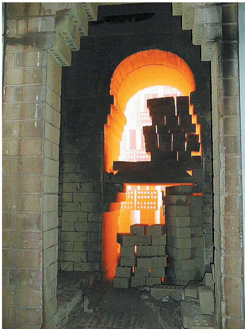
Figure 35. Relief port door in a brick manufacturing kiln (courtesy of Midland Brick Company)
