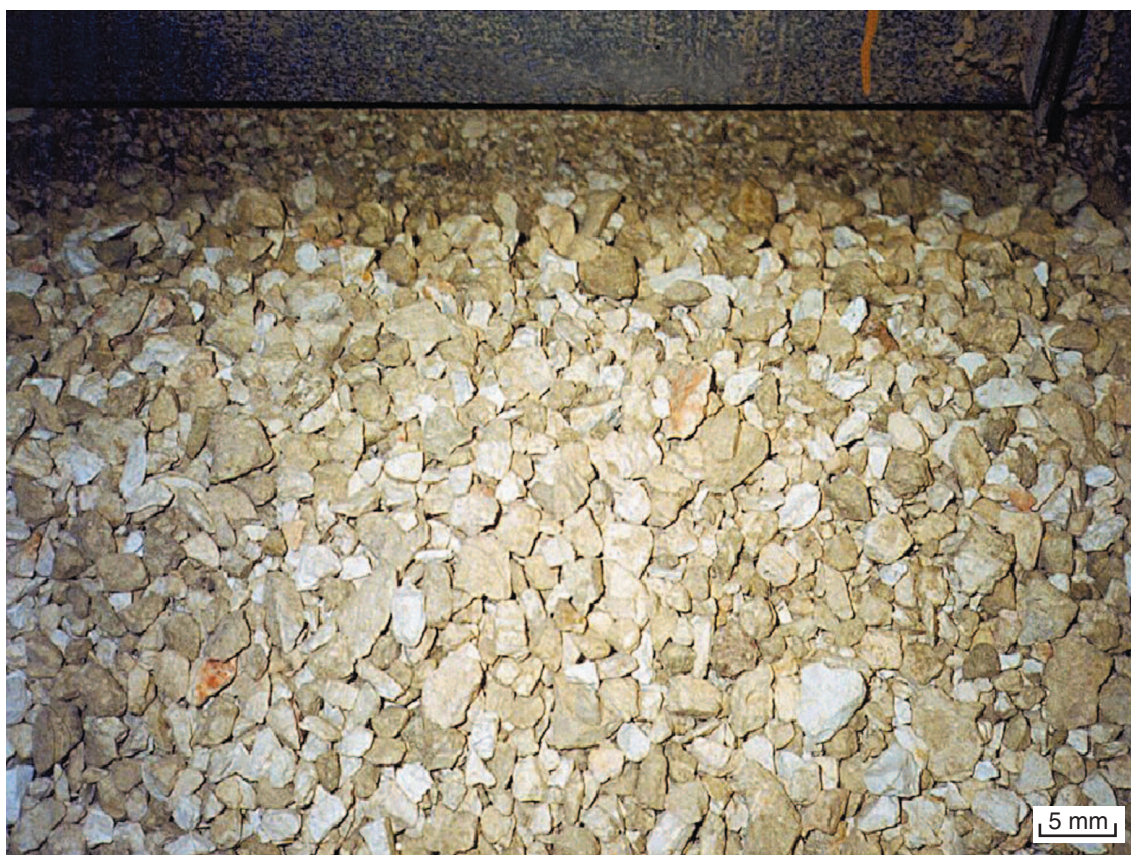
Figure 33. Milled attapulgite in the plant at Narngulu, near Geraldton
