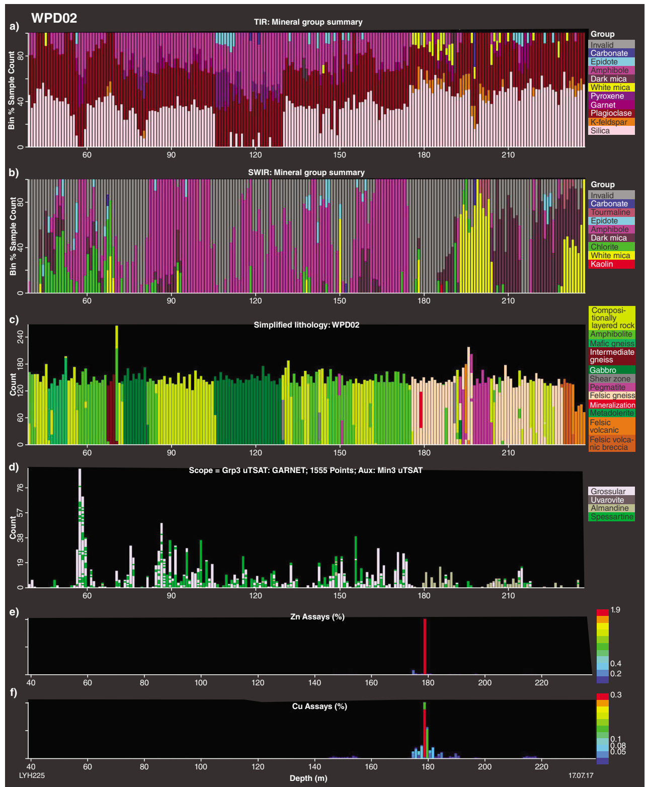
Figure 18. HyLogger, lithology and assay data for WPD02: a) TIR group summary; b) SWIR group summary; c) simplified log; d) downhole distribution of garnets (TIR mineral 3); e) % Zn; f) % Cu
