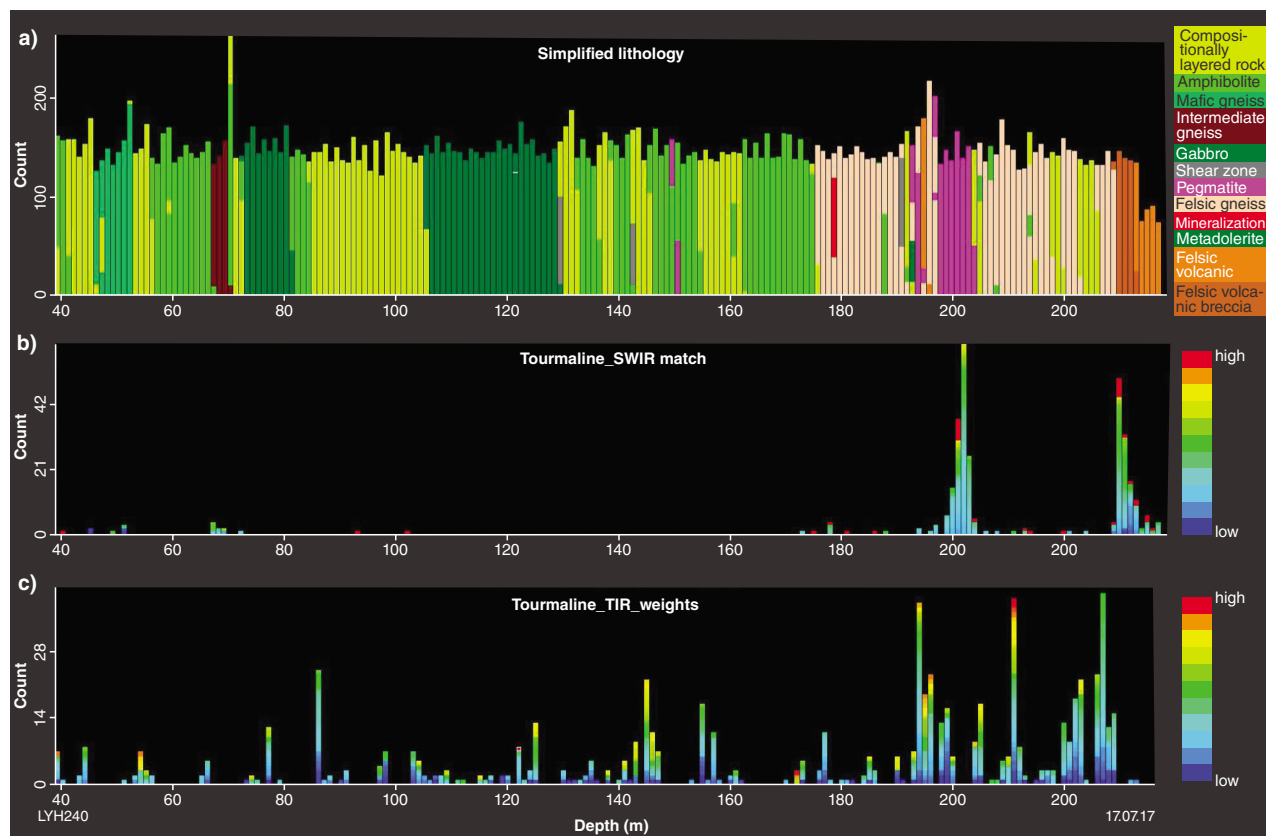
Figure 33. Weighted downhole distribution of tourmaline in WPD02: a) simplified log; b) SWIR spectra; c) TIR spectra
