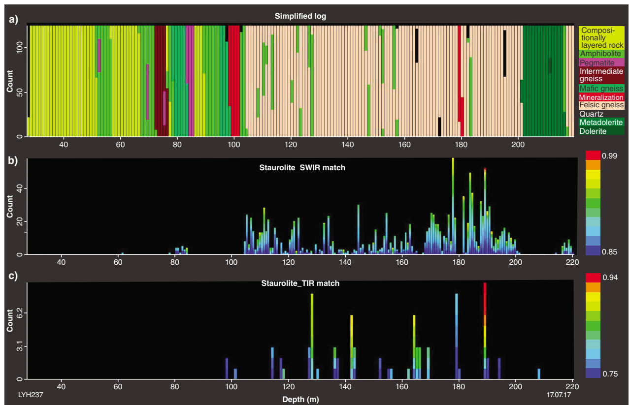
Figure 30. Downhole match for staurolite in WPD04 with SWIR spectra of staurolite from the United States Geological Survey (USGS) spectral library and with the TIR spectra from the John Hopkins University (JHU) spectral library vs simplified log
