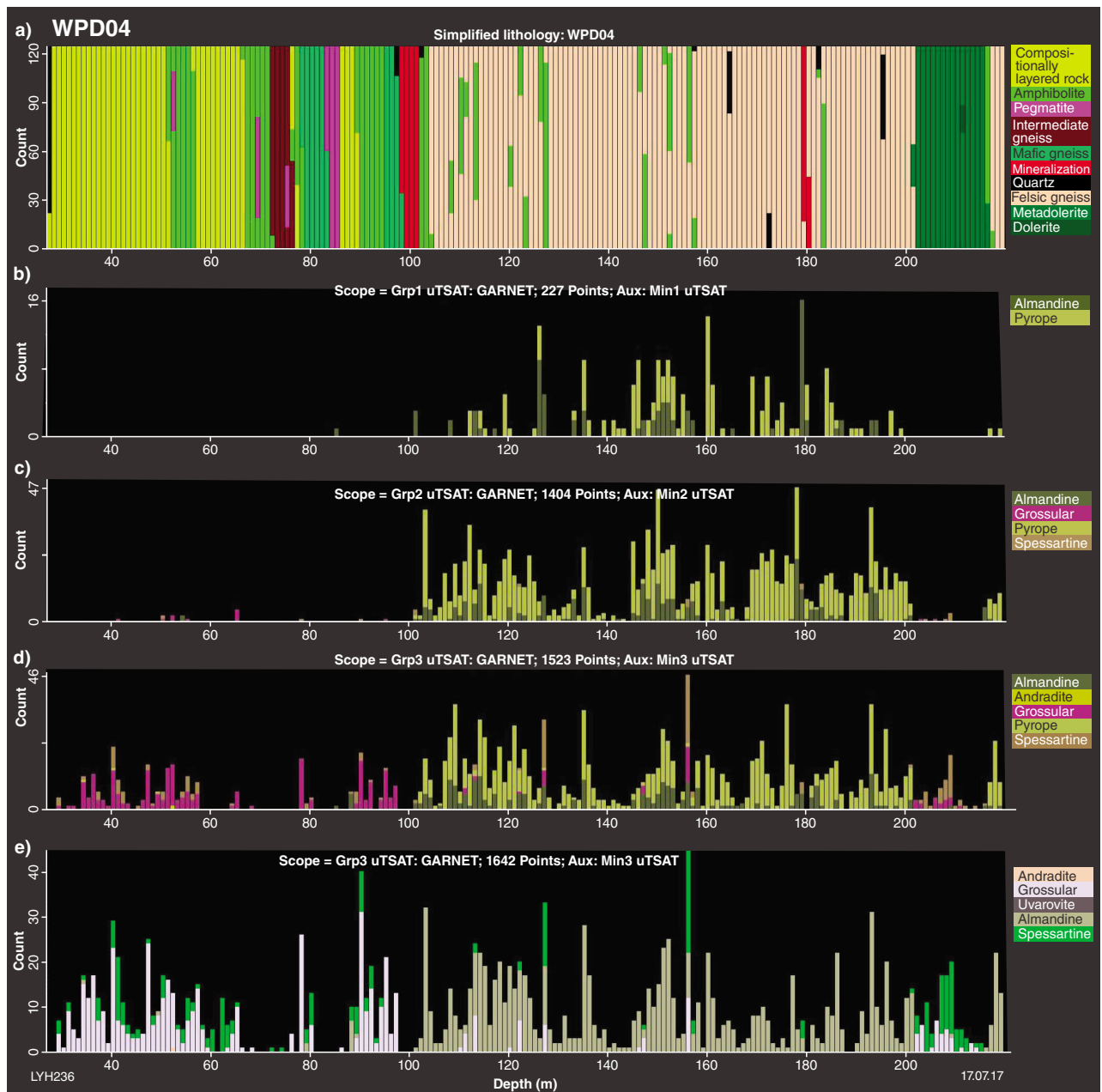
Figure 29. HyLogger interpretations of variation in garnet composition downhole vs simplified log for WPD04: a) simplified log; b) garnet as mineral 1, TSG v7.1.0.049; c) garnet as mineral 2, TSG v7.1.0.049; d) garnet as mineral 3, TSG v7.1.0.049; e) garnet as mineral 3, TSG v7.1.0.062
