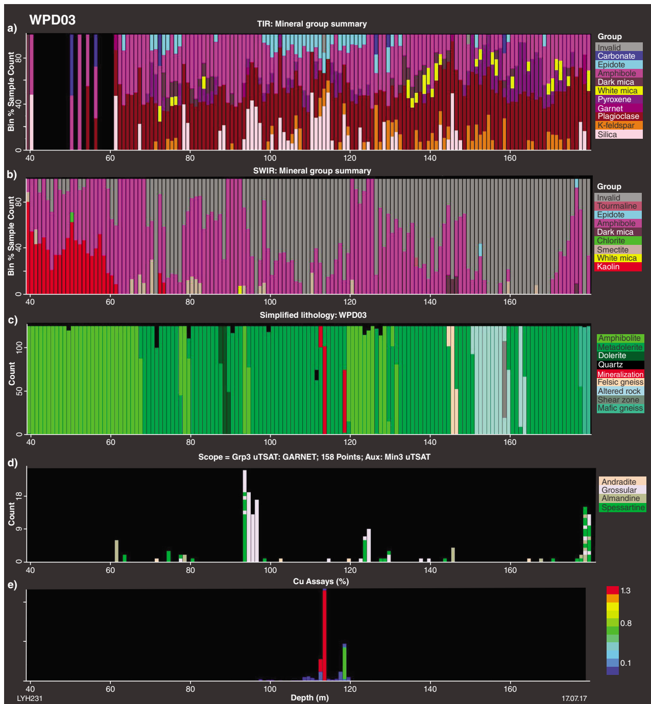
Figure 24. HyLogger, lithology and assay data for WPD03: a) TIR group summary; b) SWIR group summary; c) simplified log; d) downhole distribution of garnets (TIR mineral 3); e) % Cu
