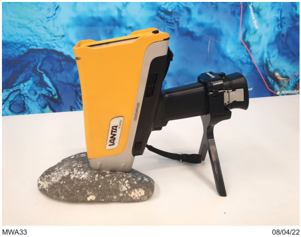
Figure 1. Olympus Vanta M-Series portable XRF analyser with soil foot attachment
