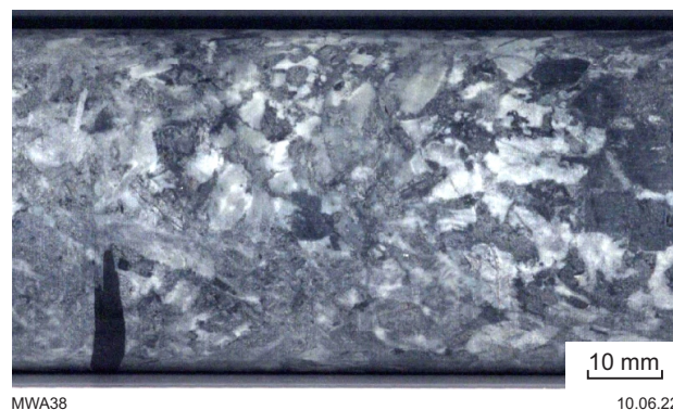
Figure 6. Coarse-grained (5–7 mm) intermediate igneous intrusion from 215 m in drillcore 18JBDD002 (M0002838) from the Jimberlana dyke intrusion, composed primarily of plagioclase, pyroxene, chlorite, white mica, and minor quartz
