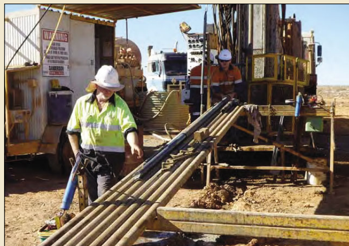
Figure 2. Diamond drill rig in operation at site MAD014 showing solid HQ core being extracted from the tube
