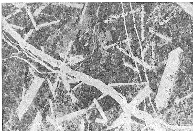
Fig. 13. Microcrystalline and sparry quartz pseudomorphing gypsum in silicified siltstone ('chert'). Jillawarra, J14, 48541, 231.1 m. Field of view 10.5 mm. (Thin section, plane polarized light.)
