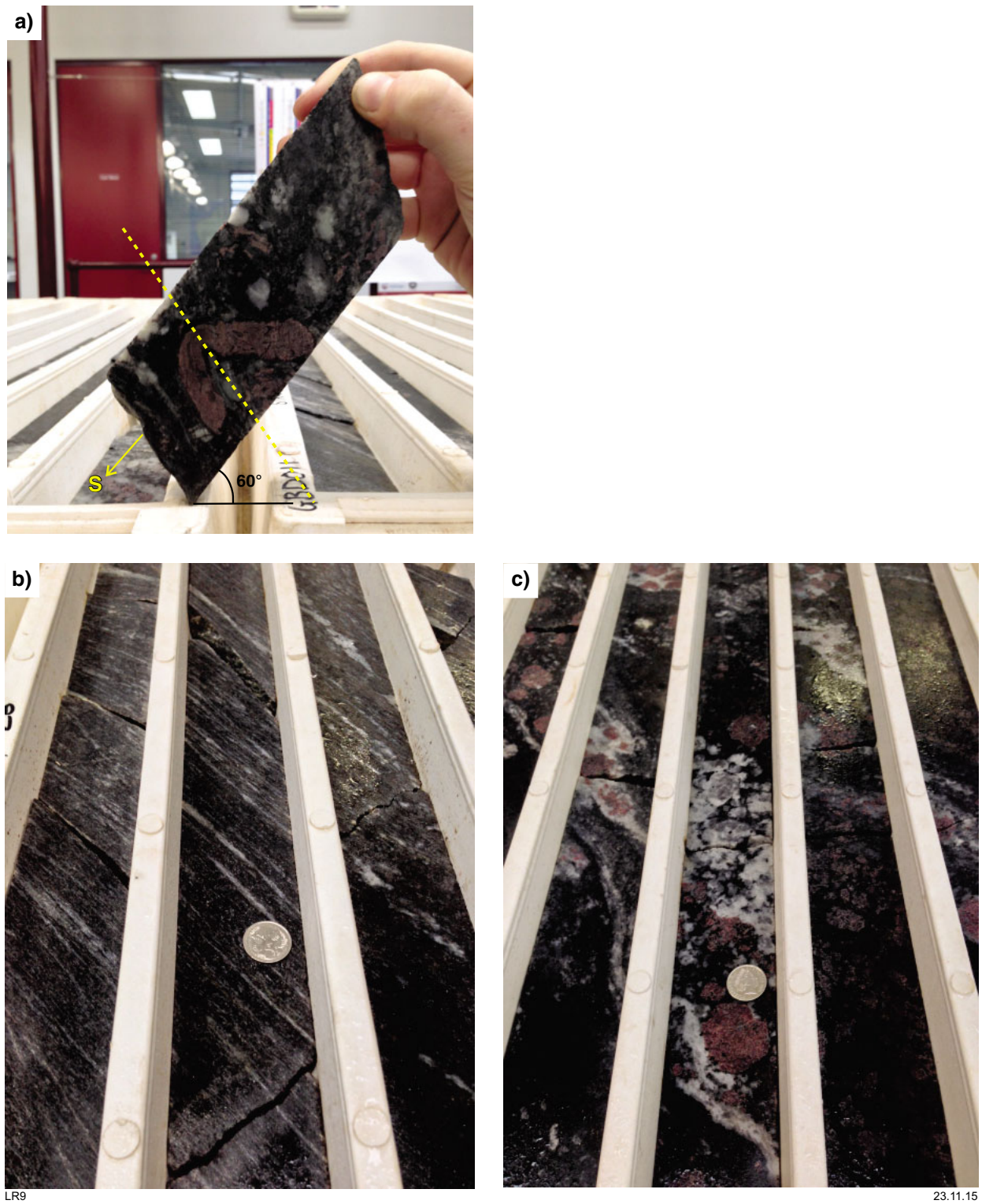
Figure 10. Oriented drillcore (5 cm diameter) with folded garnet aggregates and migmatites deformed to varying levels of strain: a) orientated core (plunging 60° towards 185°; GBD011 222.3 – 222.4 m) with a folded garnet aggregate; gneissic layering dips north; b) highly strained and stretched biotite–quartz–feldspar gneiss (GBD011 291–293 m); c) weakly deformed biotite–quartz–feldspar gneiss; quartz and feldspar clasts are coarse and show little evidence of stretching (GBD011 178 – 180.5 m)
