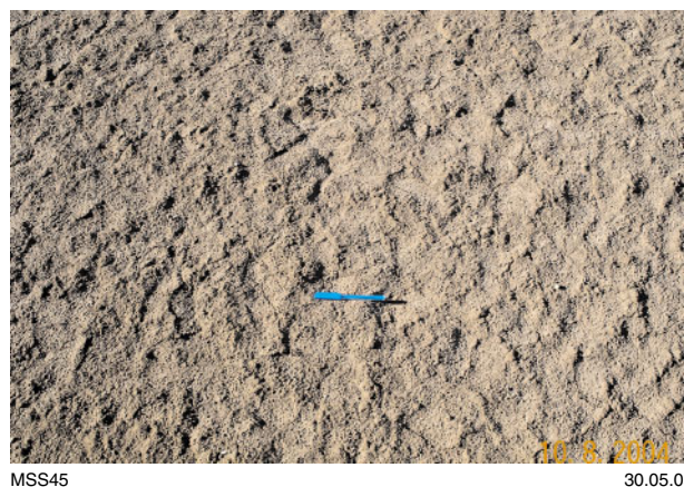
Figure 3.49. Orange-brown sandy-clay playa surface with rare fine-grained quartz and ferruginous pisoid lag. Sample site 255874; length of pen is 13.5 cm
