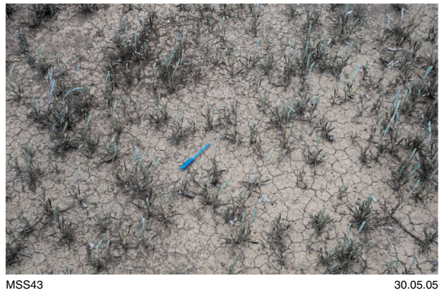
Figure 3.43. Mud cracks in sandy clay in drainage. Sample site 257332; length of pen is 13.5 cm
