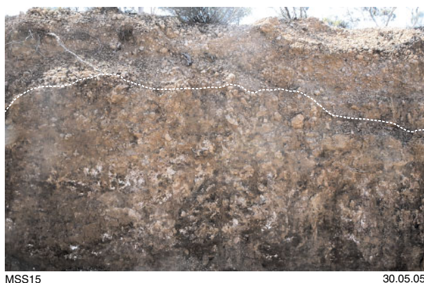
Figure 3.1. Close-up of nodular calcrete ( R k ) overlying cemented ferruginous gravel. Sample site 255777 (343755E 6622685N)
