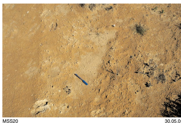
Figure 3.55. Gypsiferous crust and rare quartz lag on surface of gypsiferous sand dune. Sample site 255795; length of pen is 13.5 cm
